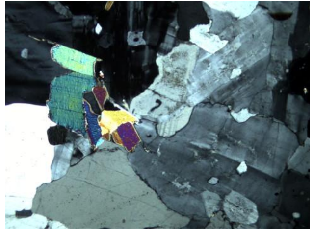
General view: Holocrystalline seriate texture with feldspar, quartz, plagioclase and muscovite.
