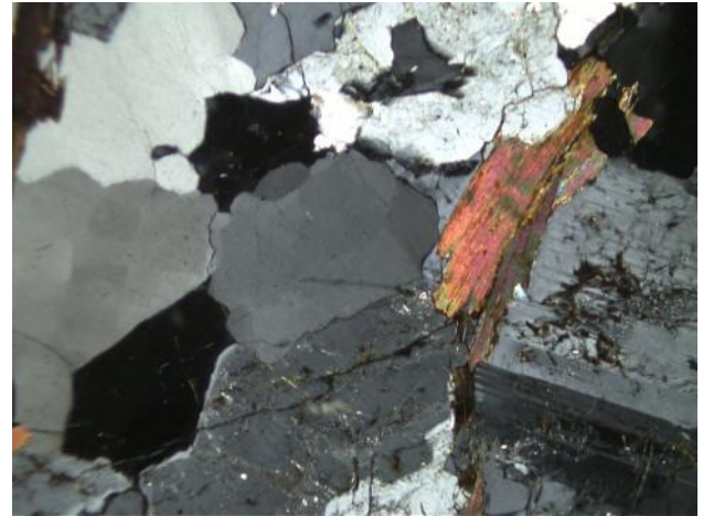
General view: Holocrystalline seriate texture with feldspar, quartz, plagioclase and biotite. Sericite, saussurite (on feldspar and plagioclase) and chlorite (on biotite) are also present.
