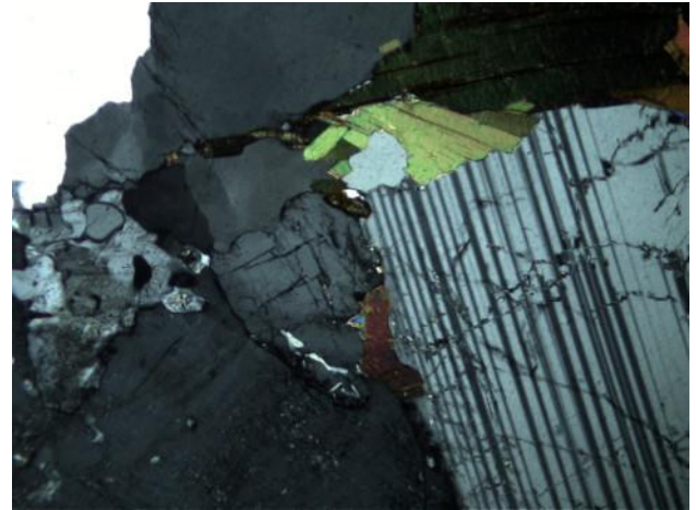
General view: Holocrystalline seriate texture with plagioclase, quartz, biotite and feldspar. Sericite is also present.
