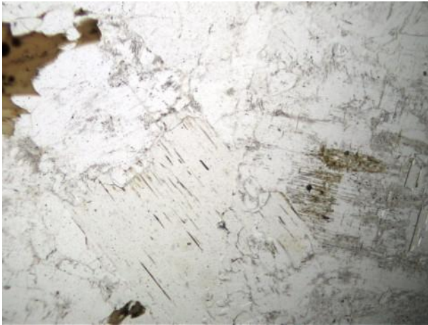
General view: Holocrystalline seriate texture with feldspar, quartz, plagioclase, muscovite and biotite. Sericite is also present.
