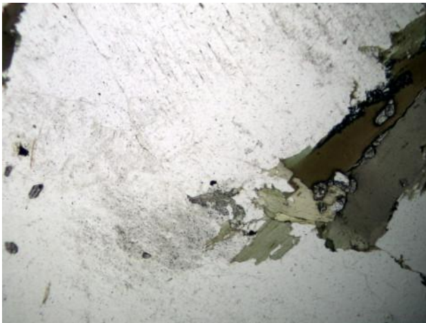
General view: Holocrystalline seriate texture with plagioclase, quartz, biotite and feldspar. Zircon and sericite are also present.
