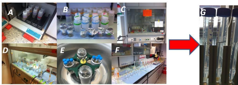
Fig. 2.3.4.1- Samples preparation: (A, B) quartz extraction, (C) quartz dissolution with HF and \text{HNO}_3 , (D) anion columns, (E) centrifuge, (F) oxalic columns and final Beryllium samples.
