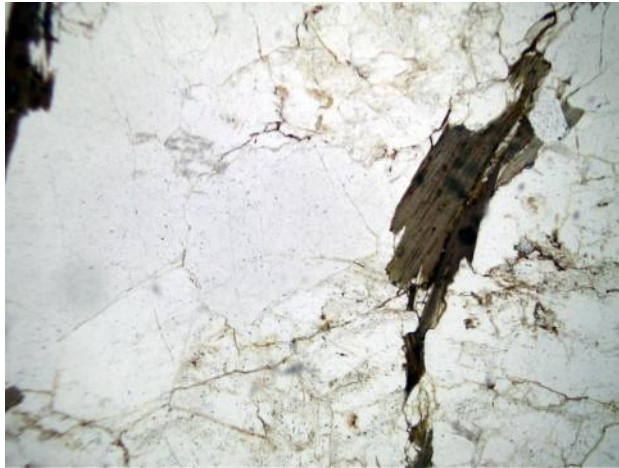
General view: Holocrystalline seriate texture with feldspar, quartz, plagioclase and biotite. Sericite, saussurite (on feldspar and plagioclase) and chlorite (on biotite) are also present.
