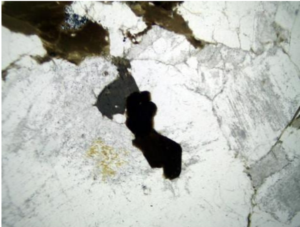
General view: Holocrystalline seriate texture with plagioclase, quartz, biotite. Tourmaline, sericite and saussurite are also present.
