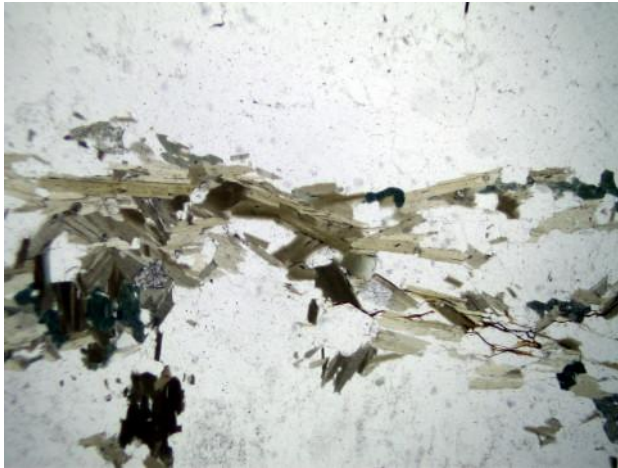
General view: Holocrystalline seriate texture with feldspar, quartz, plagioclase, amphibole and biotite. Sericite and chlorite are also present.
