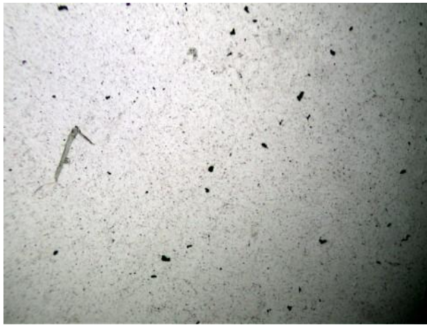
General view: granoblastic layers (quartz) with subordinate chlorite.
