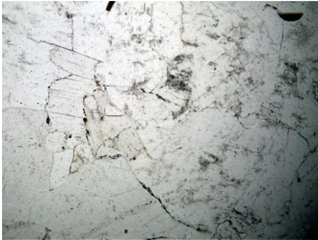
General view: Holocrystalline seriate texture with feldspar, quartz, plagioclase and muscovite.
