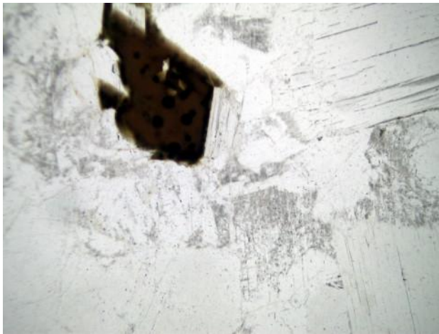
General view: Holocrystalline seriate texture with feldspar, quartz, plagioclase biotite and muscovite. Sericite (on feldspar and plagioclase) and chlorite (on biotite) are also present.
