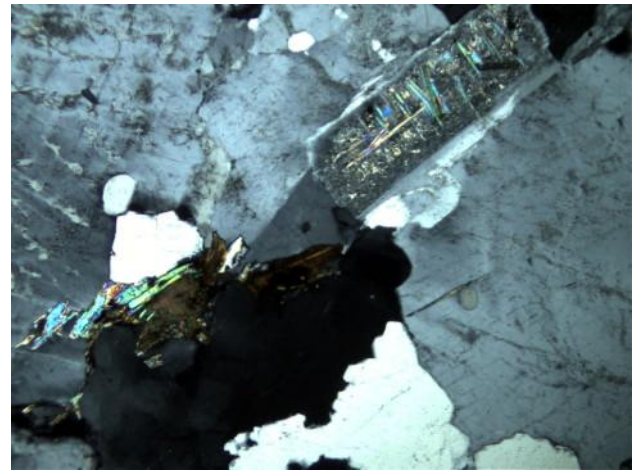
General view: Holocrystalline seriate texture with feldspar, quartz, plagioclase, biotite and muscovite. Sericite and chlorite are also present.
