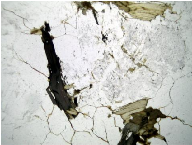
General view: Holocrystalline seriate texture with feldspar, quartz, plagioclase and biotite. Sericite and muscovite (on feldspar) are also present.
