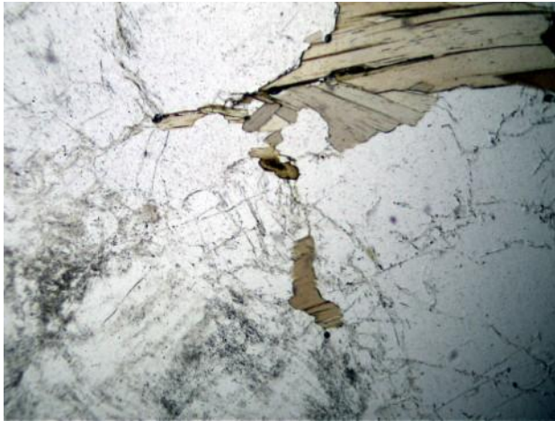
General view: Holocrystalline seriate texture with plagioclase, quartz, biotite and feldspar. Sericite is also present.
