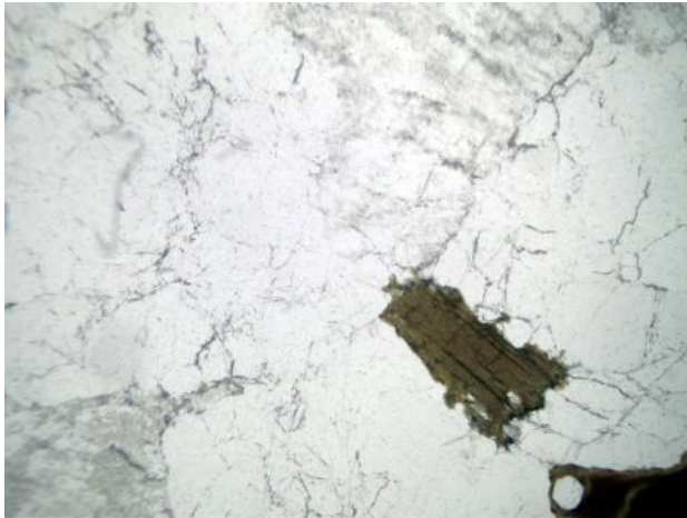
General view: Holocrystalline seriate texture with feldspar, quartz, plagioclase and biotite. Apatite and sericite (on feldspar) are also present.
