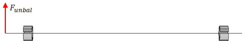
Figure 7.16: Unbalance load on the rotor end
