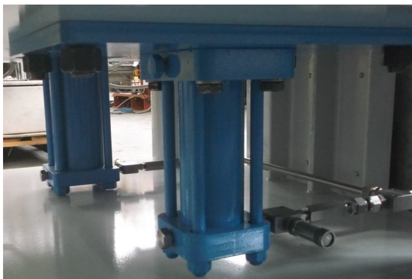
Figure B.8: View of a dissipative element.
