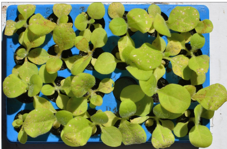
Figure 5.8 – The miniaturized kit for biomonitoring of O_3 with tobacco Bel-W3 germlings. The external dimensions are 12.5x8.5 cm. Please note necrotic lesions induced by the exposure to ambient air in the presence of O_3 .
