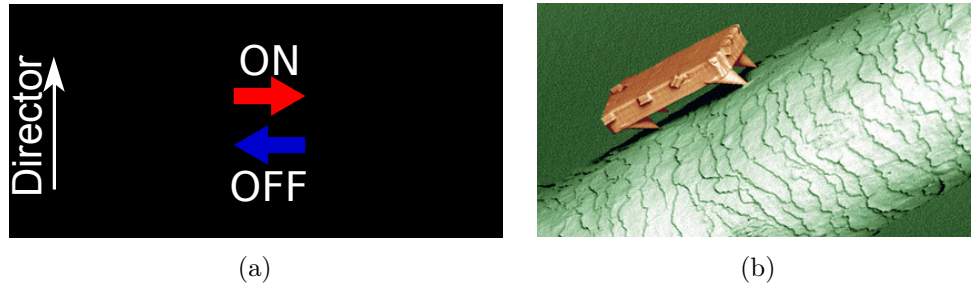
Fig. 1.4: (a) LCE molecule nematic network on the left. With an external stimulus (temperature, light, electric field..), the material contracts along the director and expands in the perpendicular plane elastically. It recovers the initial shape, once the stimulus is turned off. (b) An example of a LCE micro-robot (Image from the cover page of Adv. Mat. 27, 26 (2015)).
