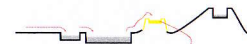
Proposed water system, with a low storage and the use of the existing topography to create an intermediate water system. This system requires less pumping power and enables a direct discharge into the sea in occurrence of a peak event.
