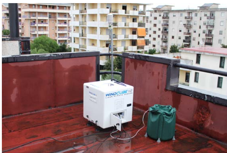
Figure 5. WindCube V2 installation.
