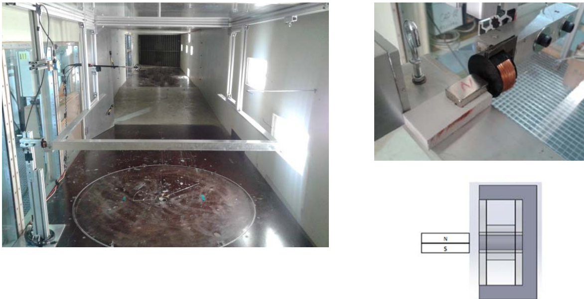
Figure 2. Horizontal set-up installed in the test section (left) - Coil/magnet assembly (right)
