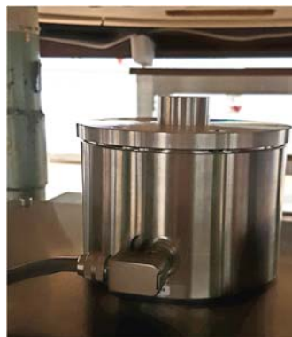
Figure 2. Schematic representation of a pressure sensor (left), and a high-frequency balance for the measurement of the base bending moment as well as of integral shear forces (right)
