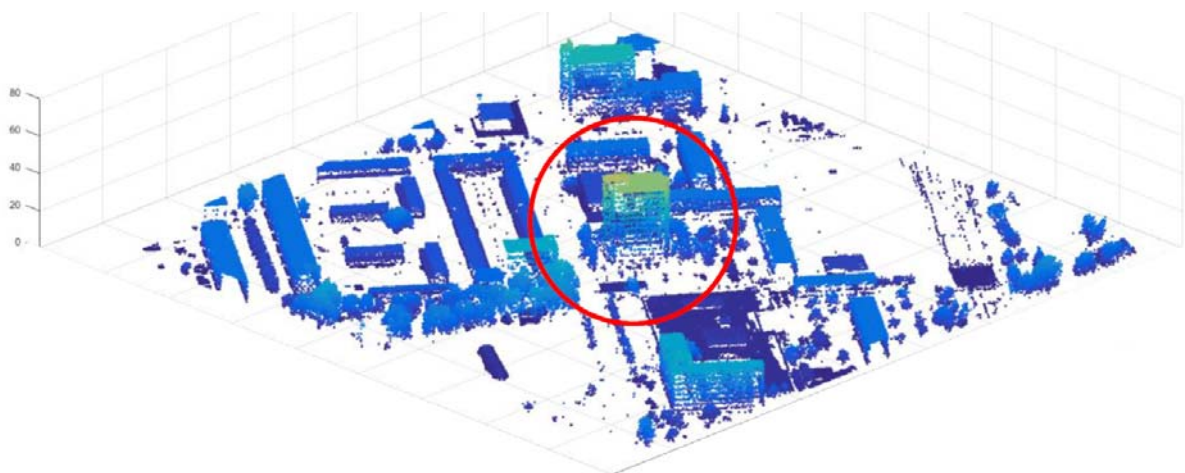
Figure 2. Example of Matlab output: Building and it's surroundings after noise reduction
