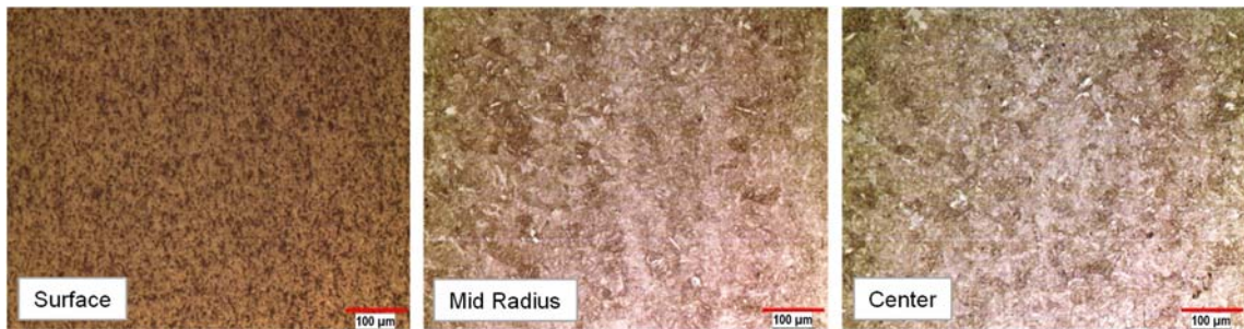
Figure 2. Microstructures (100X) from the surface to the center of the bar, 32CrB4 EXTREME Q&T Ø 56 mm.
