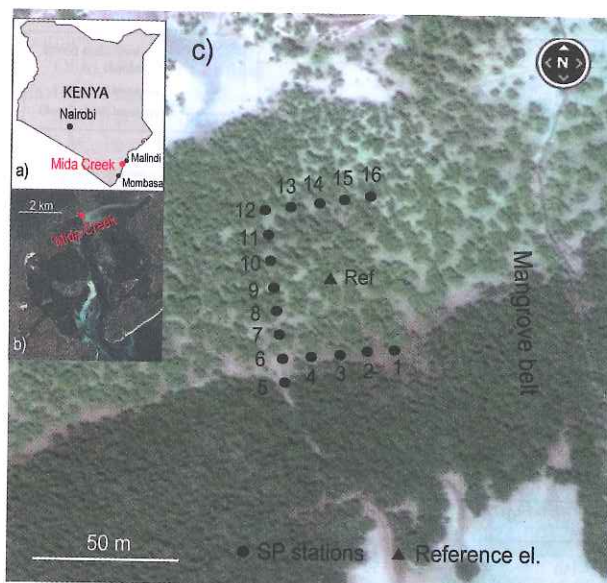
Fig. 2 – The test area in Kenya, about 25 km south of Malindi (a) in the north-western margin of Mida Creek (b); c) the C-shaped self-potential array.
