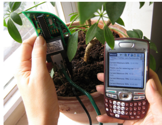
Fig. 3.3 - Botanicals: Sensori + scheda arduino + smartphone Treo.
