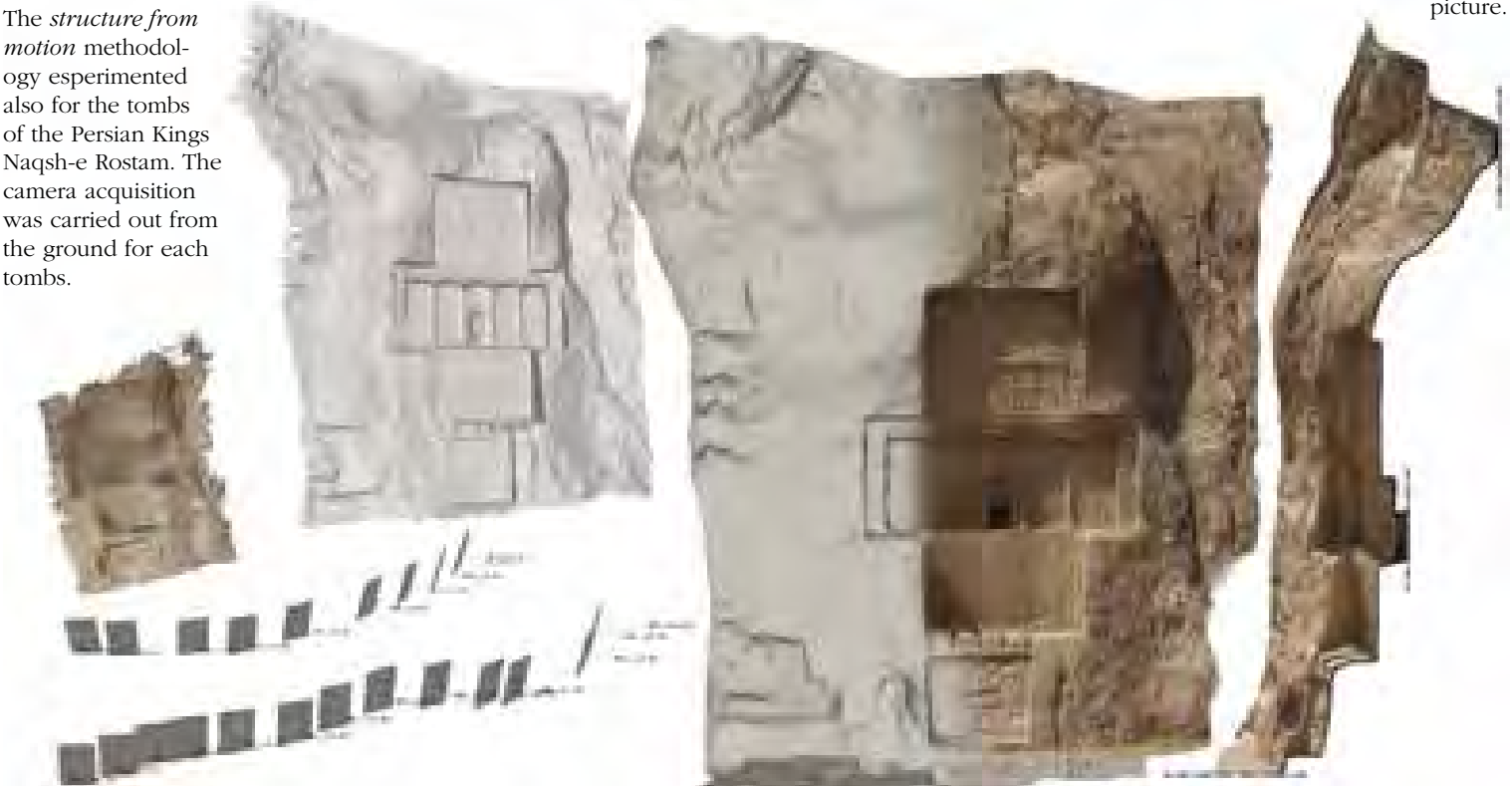
Survey methodology for all the graves. First sequence close to the tombs and the second sequence from the upper level to a overall picture.
