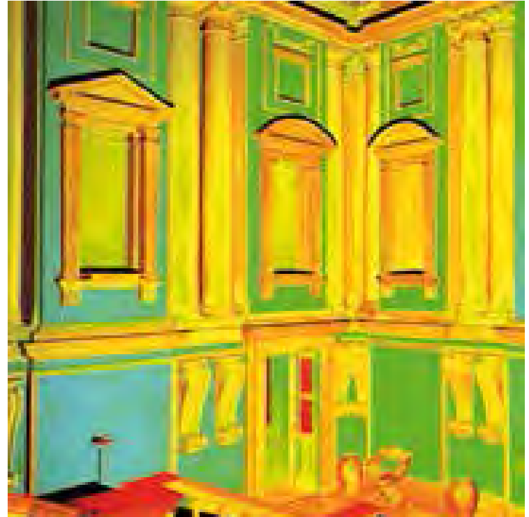
Laser scanner survey of the atrium of the library. On the right a point cloud view and the bidimensional metric front of the atrium.
