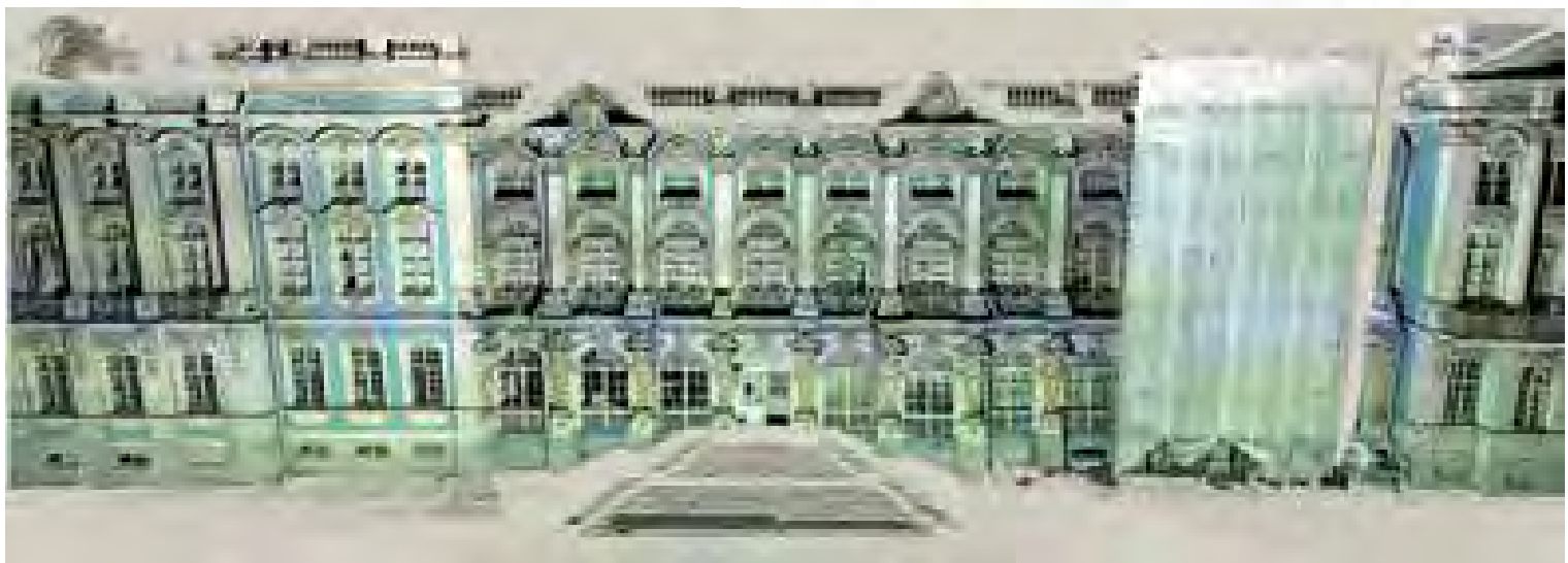
Beside: The cloud of points relative to the portion of the facade detected. Under: an image scan of the facade of the palace.
