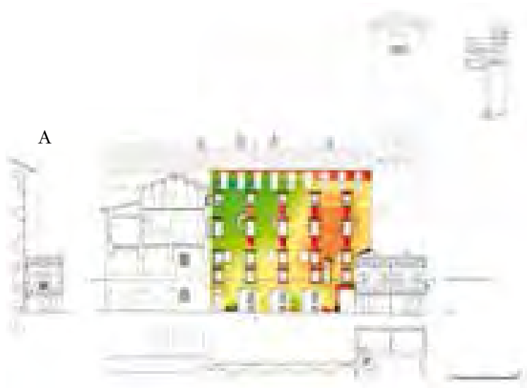
Comparison of the deformations on the facades of the palace of the Podesta. the individual surfaces are colored with a range of colors corresponding to the value of the deviation from the vertical plane of the wall.
