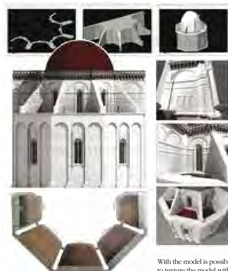
3D model process. From the general surfaces to the details of the main decorative elements.
