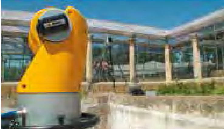
above: In the picture, the laser scanners Callidus CP3200 and Mensi GS200 work.
