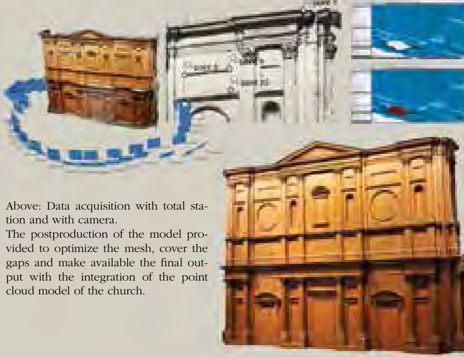
With the integration of a topographic survey and a shape from motion survey has been possible obtain a reliable and accurate 3D textured model.
