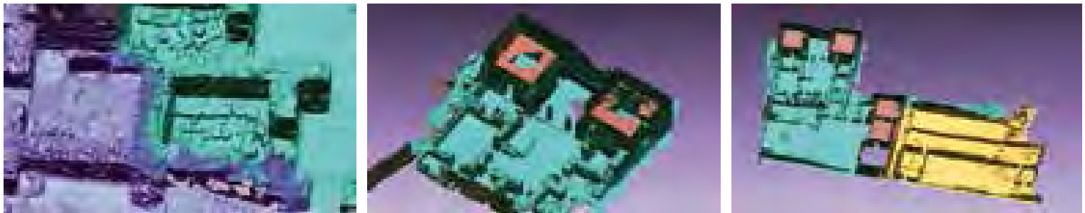
Optimization of mesh: the integration process of the gaps and the reconstruction of the missing portions of the photogrammetric model. The process has been carried out on individual three-dimensional models, subsequently combined.
