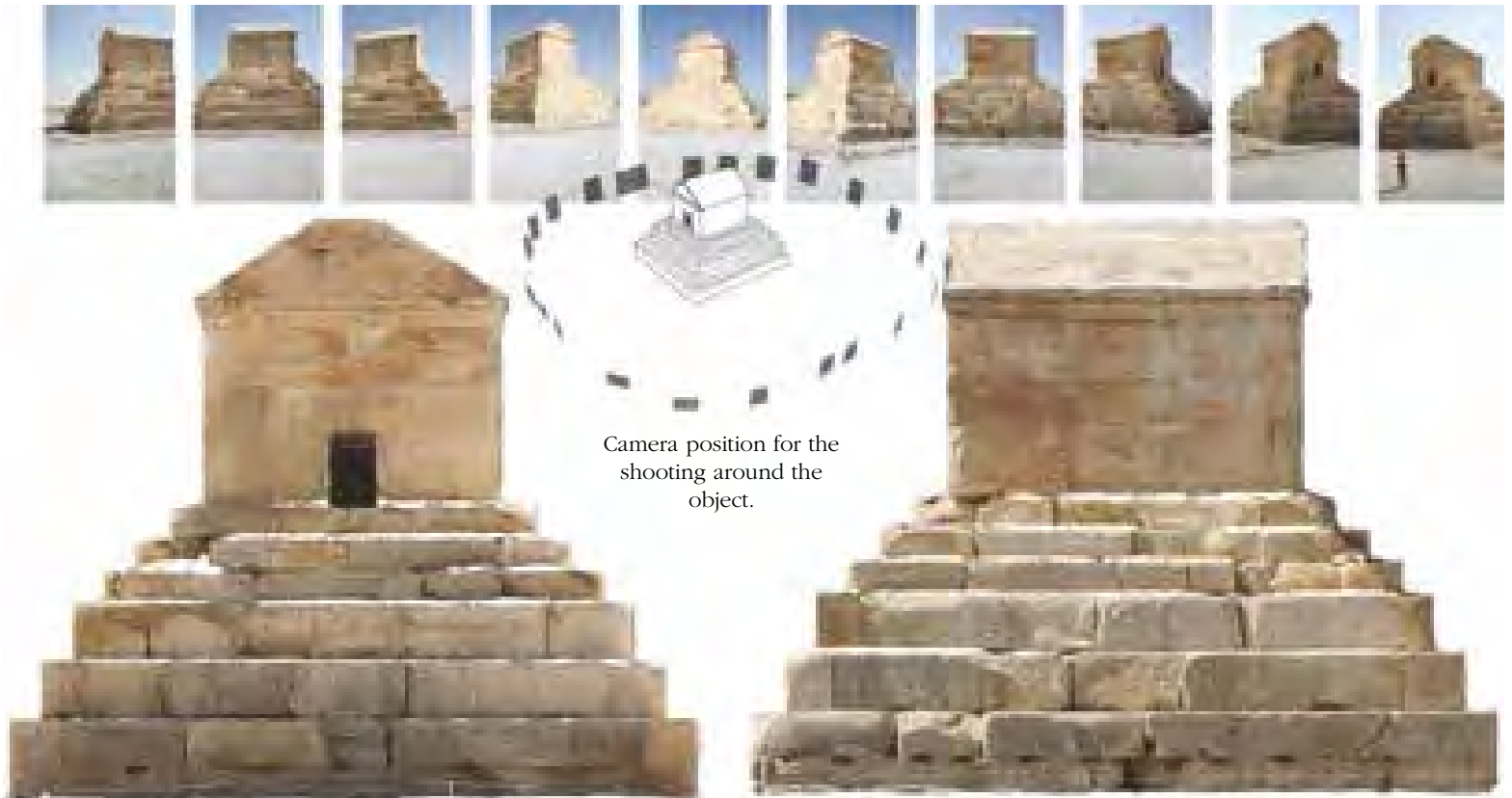
Elaboration of two-dimensional faces of the Tomb of Cyrus the Great. The model, suitably scaled on three points of the basement measured on site, has allowed to realize a photographic three-dimensional elaborate highly reliable and responsive to reality.
