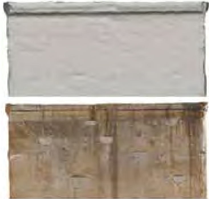
View a portion of the 3D model with and without texture. From the pattern in gray is it possible to see the characteristic of the surface discontinuities of the material obtained by this survey system. The texture gives to the model the aspects relating to the color and condition of the surface.
