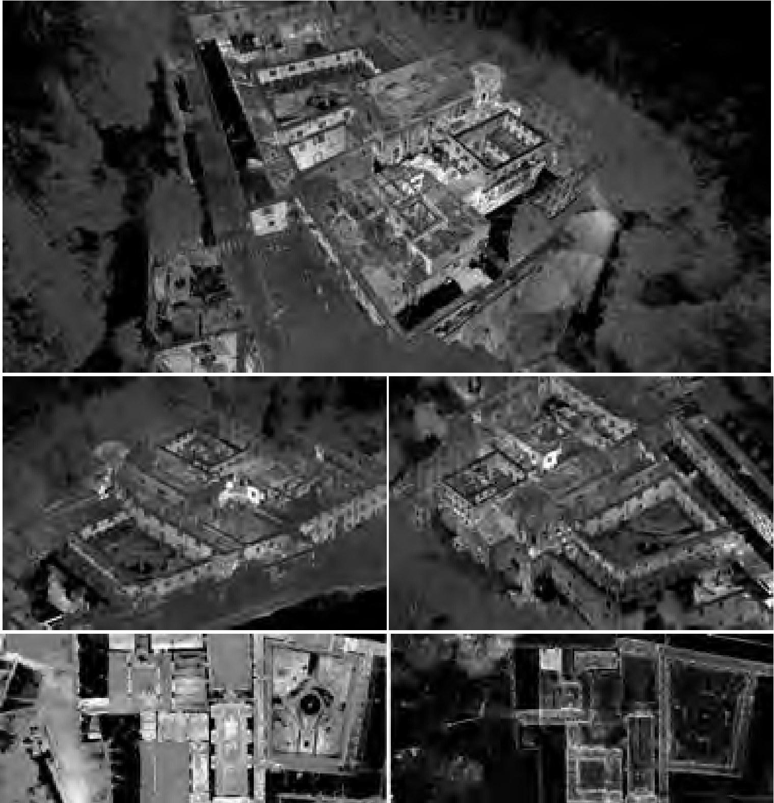
Some examples of three-dimensional databases; the point clouds acquired by laser scanner survey of complex systems: the archaeological site of Hadrian's Villa in Tivoli (Rome, Italy) examples of surveys for urban clusters of L'Aquila (Italy); and the monastery of Camaldoli (Arezzo, Italy). Through the clouds of points can be read and interpret the morphologies of the environment and the volumetric composition of space.
