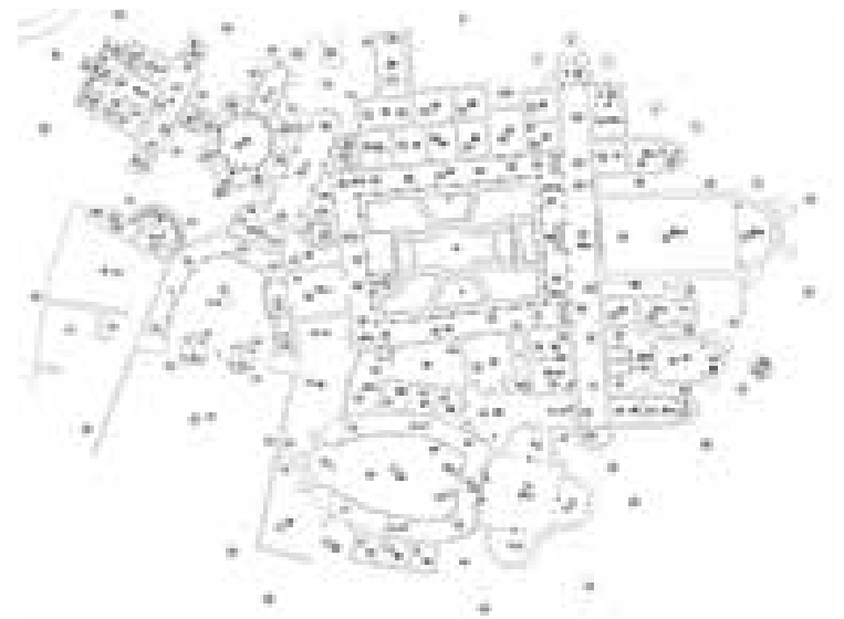
Above: the plan on the left shows the placement of the instrument laser scanner. The station points were determined in order to obtain registration of a single model.
