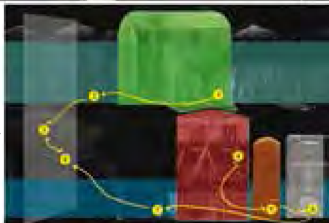
General scheme with the identification of the location and the order in which the laser scans were performed. In order to combine the laser survey of the extrados part with the intrados part it was necessary to scan at two different levels the same portion of the front facade. This was necessary to identify homologous points that led to the union of several scans.
