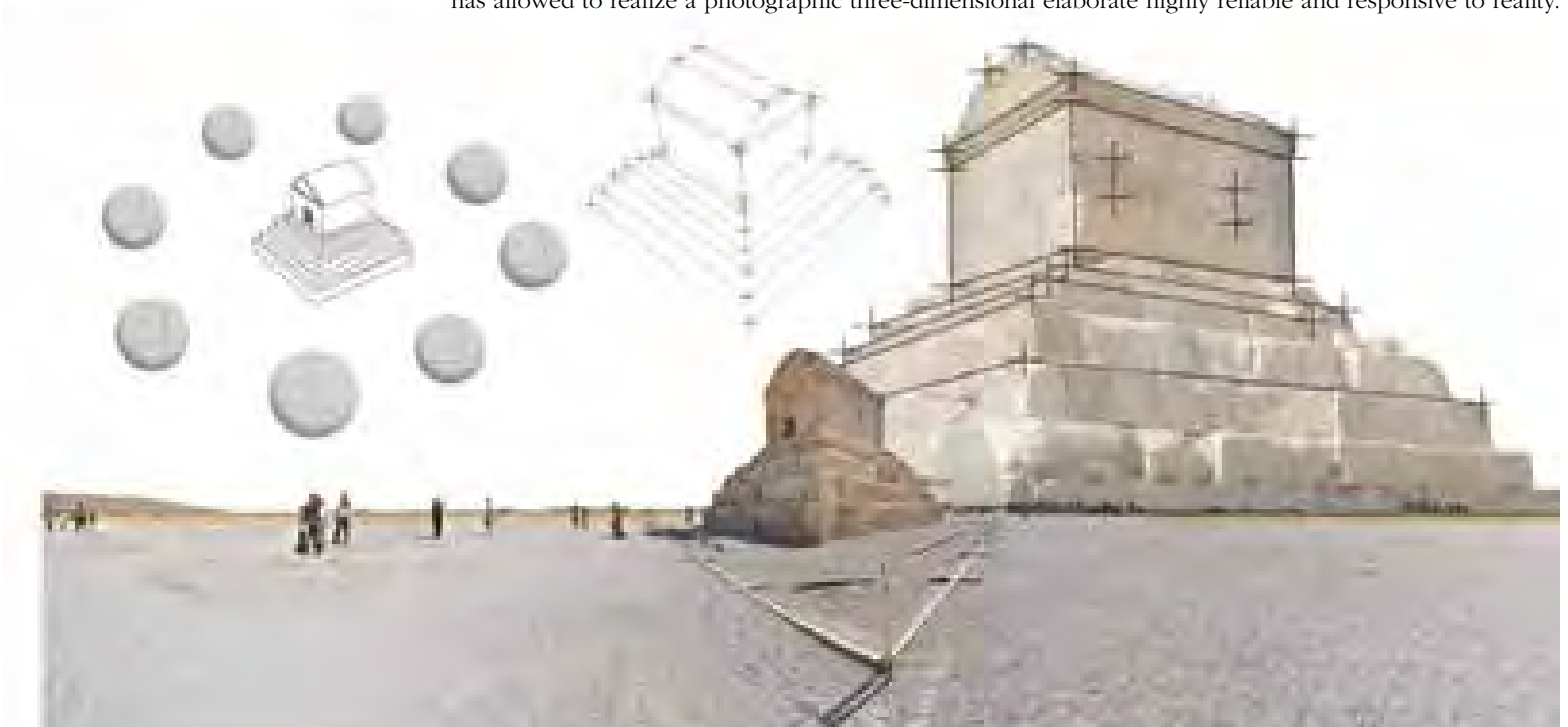
The test of reliability was performed by integrating the shape from motion survey methodology with spherical panoramas. These, surrounding the monumental building, allow to find homologous points on the object for each set of three spheres, and locate them in the tri-dimensional space using an orientation and restitution software (Shpera software, Thanks to Prof. Gabriele Fangi, University of Ancona). By overlaying the two products has been checked the reliability between the shape from motion model and the spherical model.
