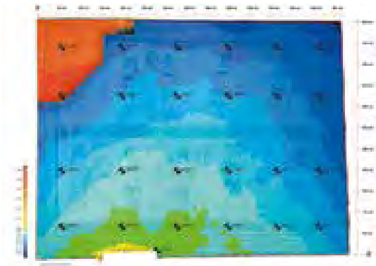
The image above proposes the study of the deviation of the plane of the mosaic floor of the room Girls in Bikinis. At the side, the orthophoto of the above flooring.
