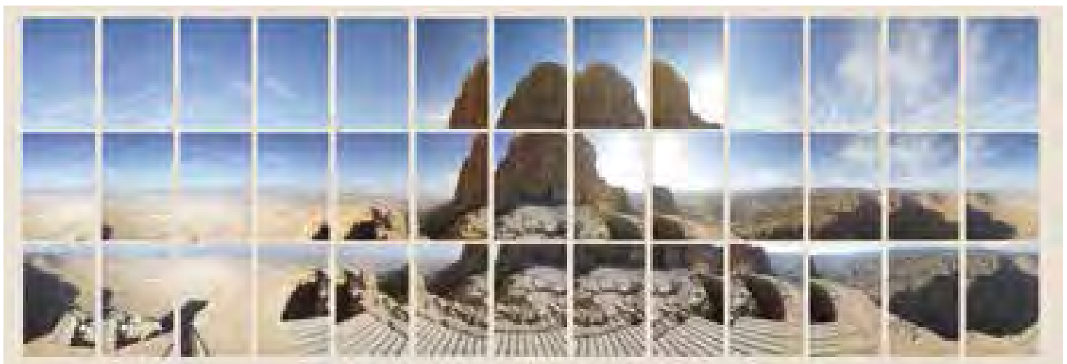
Photographic survey: on the top shape from motion methodology for the photographic acquisition. Above the panoramic view of the Masada plateau. The sequence of the pictures can generate a 360° spherical image with the observer in the middle of it. Below the movement around the object to create the right sequence of pictures that can be able to realize a 3D texture model.
