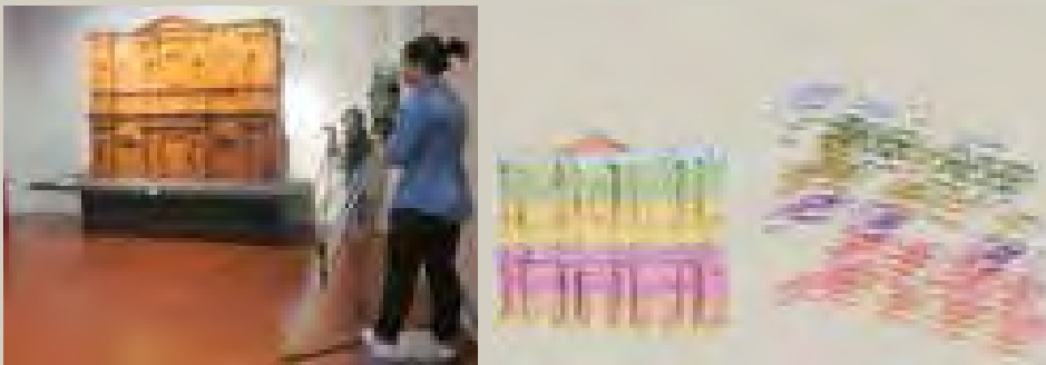
With the integration of a topographic survey and a shape from motion survey has been possible obtain a reliable and accurate 3D textured model.
