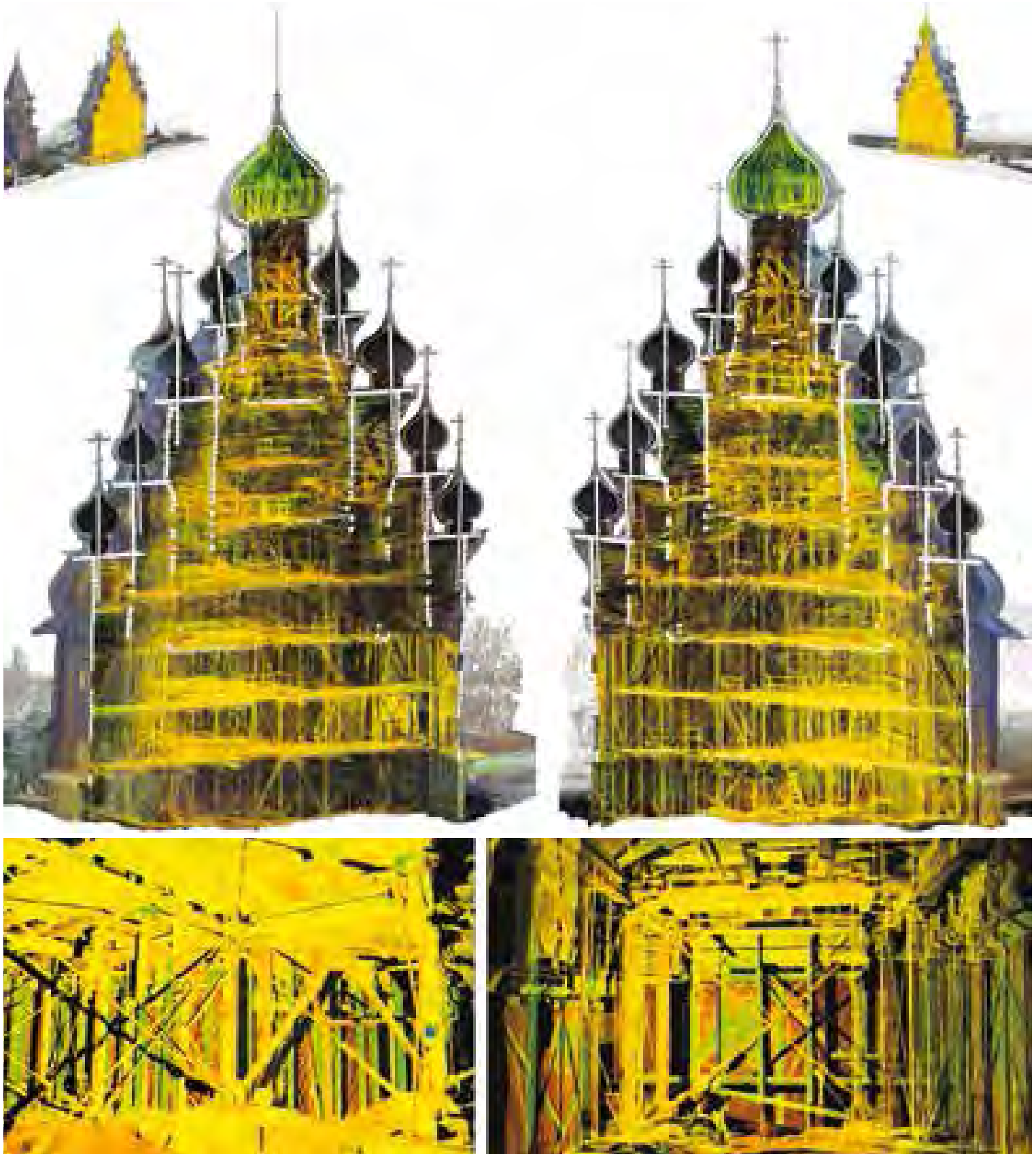
General view of the point cloud of the Church of the Transfiguration. Bottom: detail views of the point cloud of the church interior.
