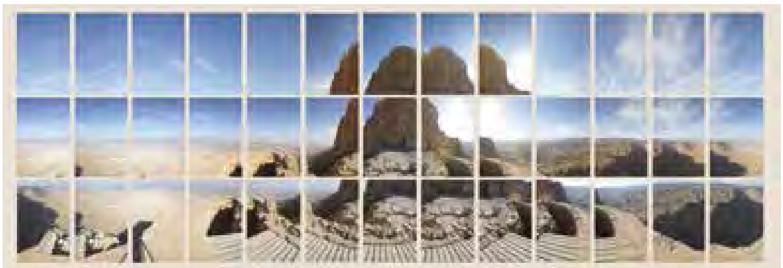
Photographic survey: on the top shape from motion methodology for the photographic acquisition. Above the panoramic view of the Masada plateau. The sequence of the pictures can generate a 360° spherical image with the observer in the middle of it. Below the movement around the object to create the right sequence of pictures that can be able to realize a 3D texturize model.
