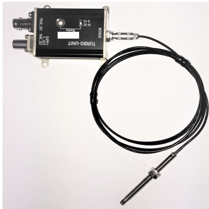
Figure 48. TC speed sensor and an electronic unit for raw signal conditioning.
