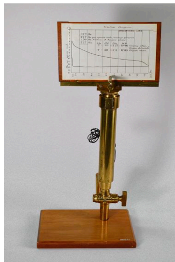
Figure 1. Replica of the original steam indicator invented in the early 18th Century by James Watt of Scotland.
