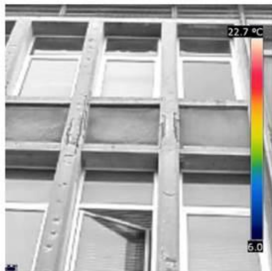
Fig 2: Carrara School: Thermal Analysis. The analysis with thermographic camera shows the presence of thermal bridges in correspondence of structural elements of the building (beams and columns)
