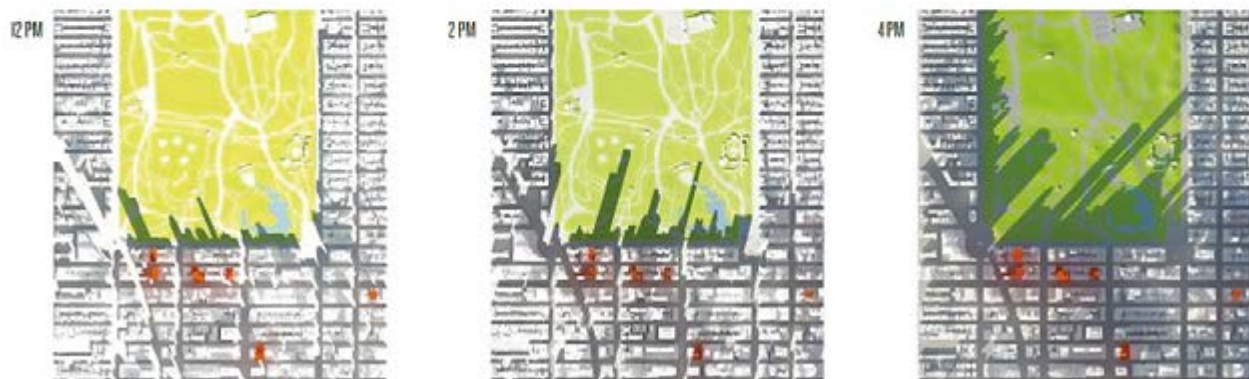
September 21st Shadows Across Central Park After Development
