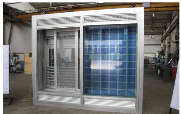
► Fig. 3: The smart façade prototype was realized by DAVINI, an Italian Tuscan company. The façade system has a thermal break frame by Schueco and glass panels by Pilkington.
