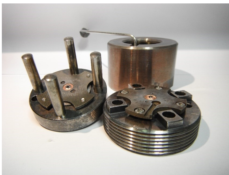
Fig. 2.13 Scheme of the Sapphire Anvil Cell (SAC).
