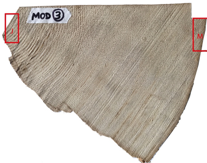
Figure 2: one of the modern wood edges used to obtain powder samples were taken both from juvenile (J) and from mature (M) wood. For modern samples both these two part has been considered as outer parts
