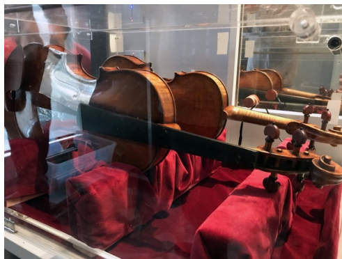
Figure 3: climatic box (T 20°C and RH 55%)
