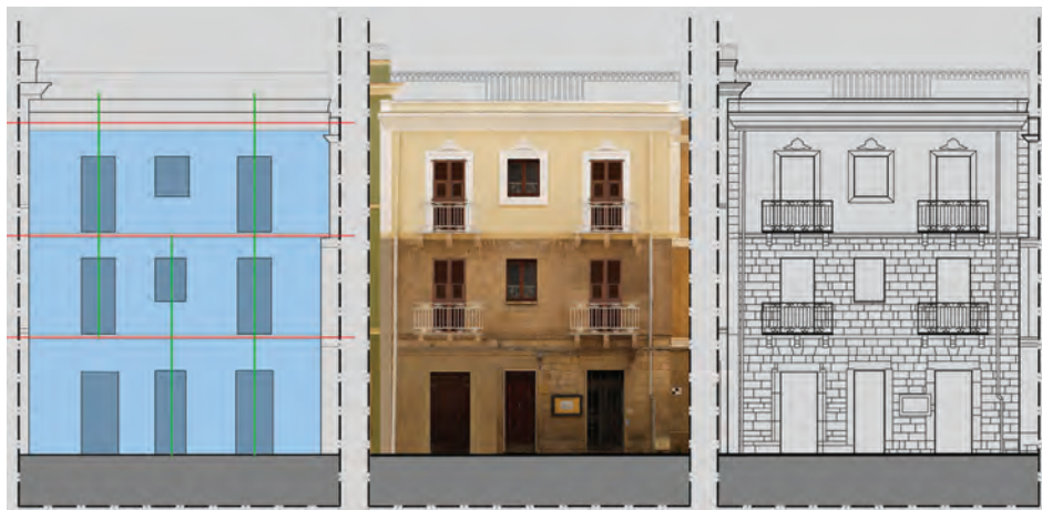
Figure 8: Graphical analysis of one of the façade surveyed in the Carloforte town center
