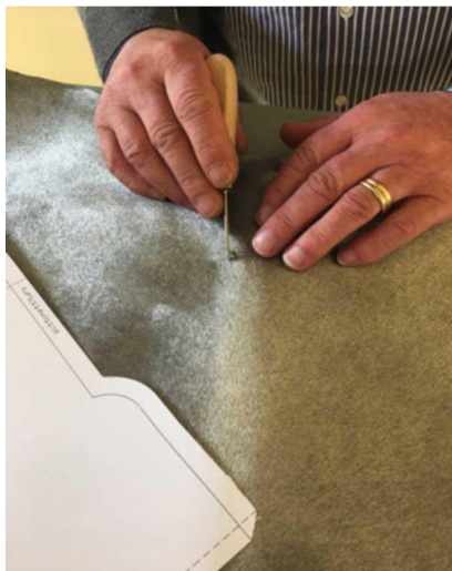
Figure. 3. Leather cutting by hand following the pattern guidelines
