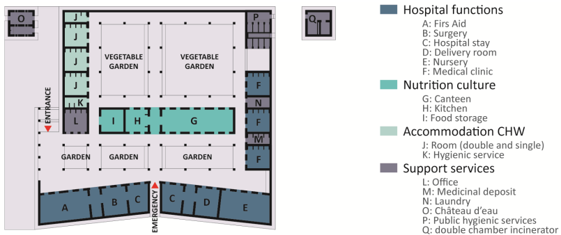
Figure 2: Functional and distribution scheme of the CSCom.
