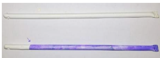
Fig. 1 MEA starter on membrane, with and without methylene blue as dye
