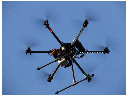
Fig. 4. Six-engine custom R.P.A.S. with thermal camera
