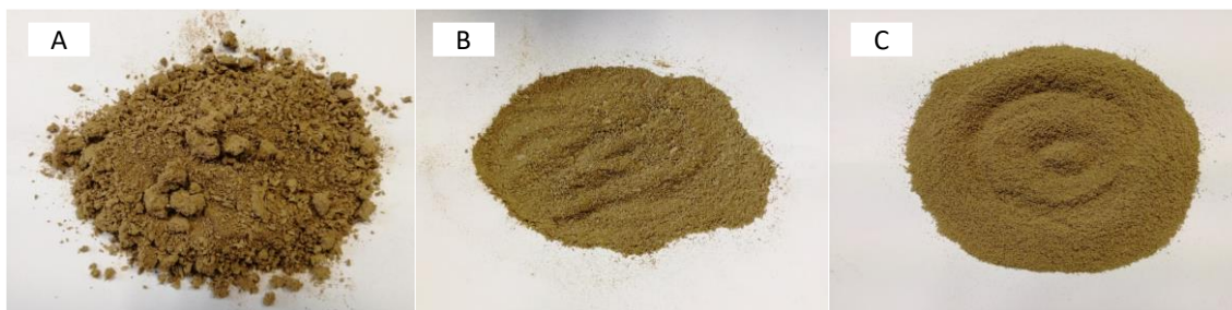
Figure 1. Dried pâté from 2016 campaign: a) dried after 18 months of storage in non-controlled conditions; b) after a rapid and preliminary grinding, 15 days after drying; c) after a rapid and preliminary grinding and sifting, 15 days after drying
