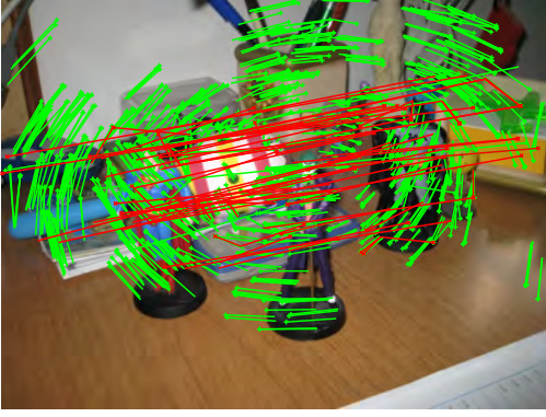
Figure 4. Flow vectors of the retained (green) and discarded (red) matches using the proposed heuristic for the sample non-planar image pair of Fig. 1 (best viewed in color).
