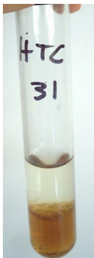
Figure 67: Extraction of an aqueous phase sample; the DEE-soluble organics are concentrated in the top-phase.
