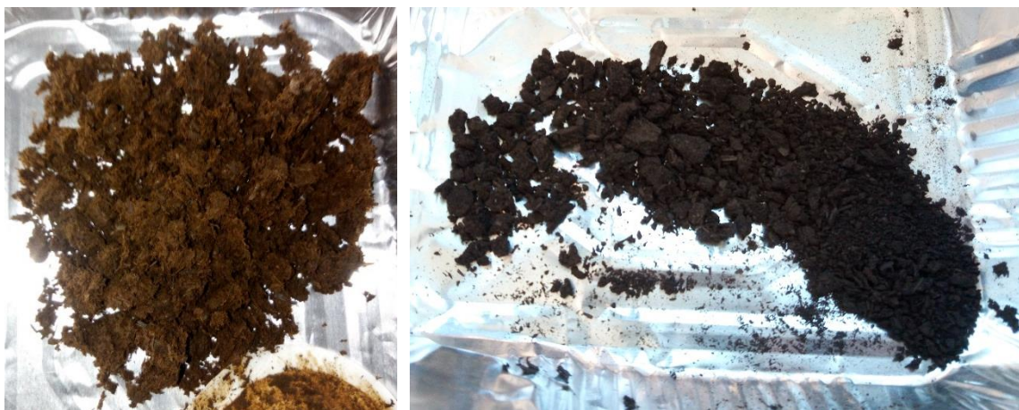
Figure 55: Comparison between hydrochar samples obtained at 3 h and different temperature: left 200 °C, right 250 °C.
