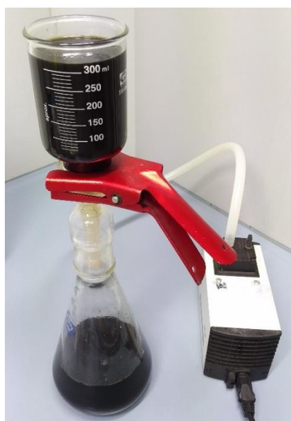
Figure 45: Vacuum filtration for solids recovery from slow pyrolysis liquid products.
