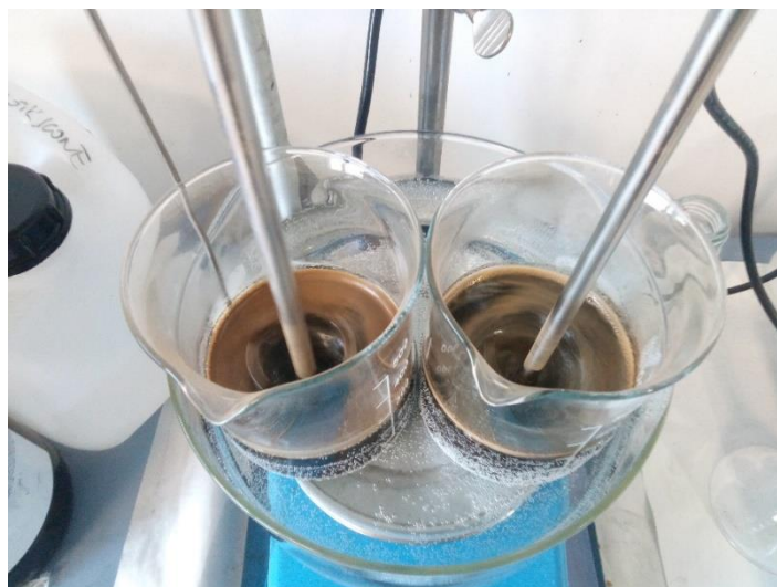
Figure 65: Impregnation of the LRR with KOH at two different mass ratios: 1:1 (left) and 2:1 (right).
