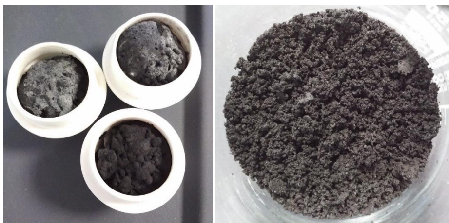
Figure 69: Chemically activated carbons from LRR; as removed from the TGA (left, the muffin effect is clearly visible) and after washing and drying (right).
