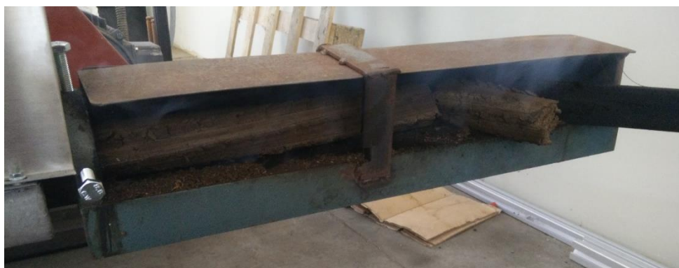
Figure 107: Dried digestate extrusion during briquetting.
