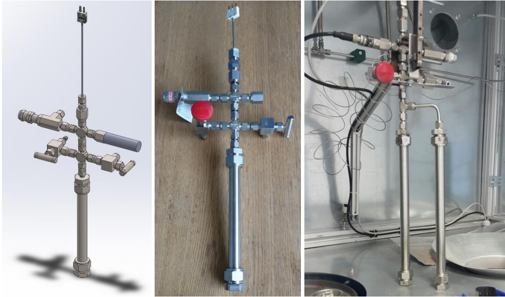
Figure 29: 3D model and picture of the reactor (single and double reactor configuration).
