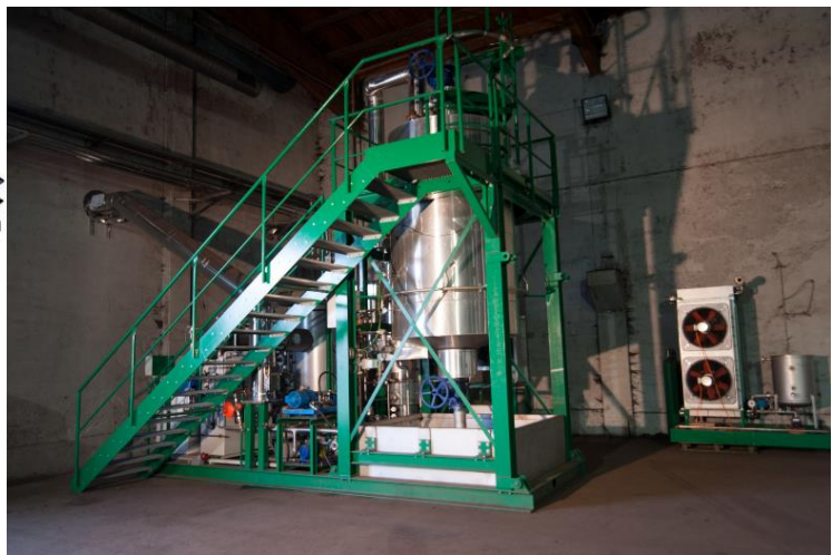
Figure 24: Representation of the SmartCarbon multi-batch HTC reactor system (left) and one HTC module in Leonberg (right) [96].
