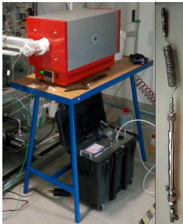
Figure 34: Horizontal tubular furnace used for activation experiments (left) and particular of the reactor (right).
