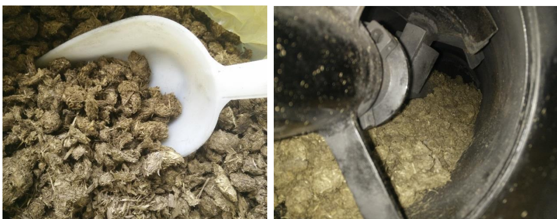
Figure 42: Batch-wise feeding of the dried digestate inside the pyrolysis reactor.
