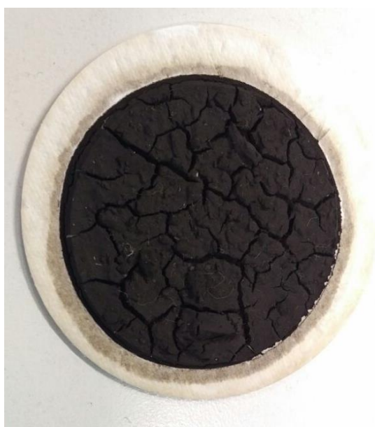
Figure 45: Vacuum filtration for solids recovery from slow pyrolysis liquid products.
