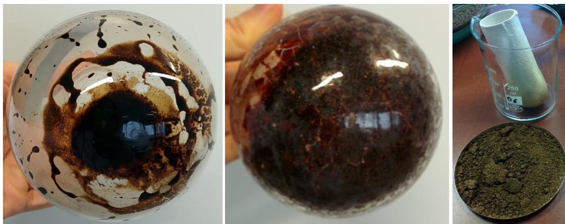
Figure 66: Water-soluble extractives (left), ethanol-soluble extractive (center) and lignin (right) obtained for the evaluation of the lignin content from the LRR.
