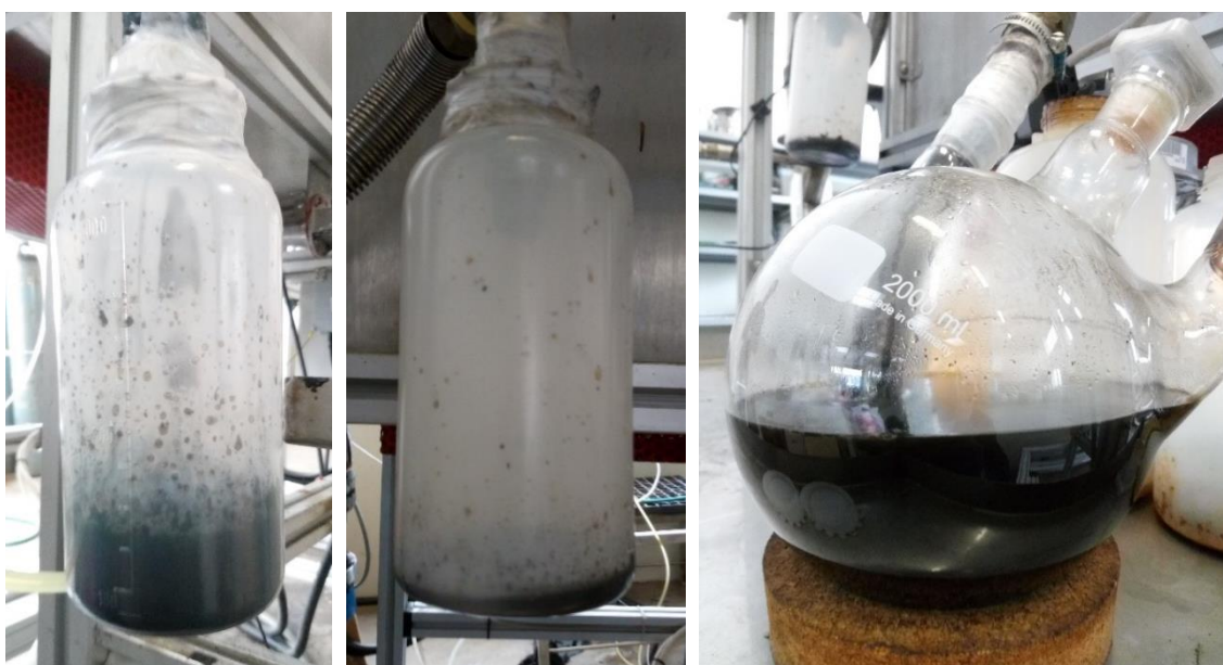
Figure 44: From left to right: condenser 1, condenser 2 and bubbler at the end of the slow pyrolysis experiment.
