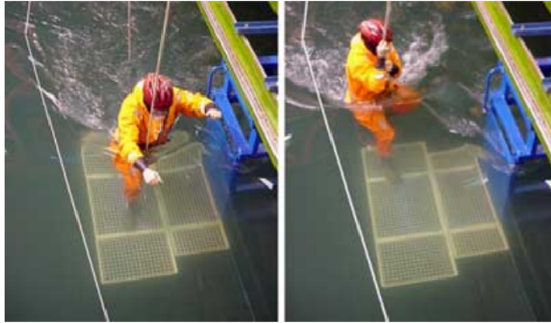
FIGURE 2.8: Experiments on human instability: water depth 1.07 m and velocity 1.0 m/s (from Karvonen et al., 2000)
