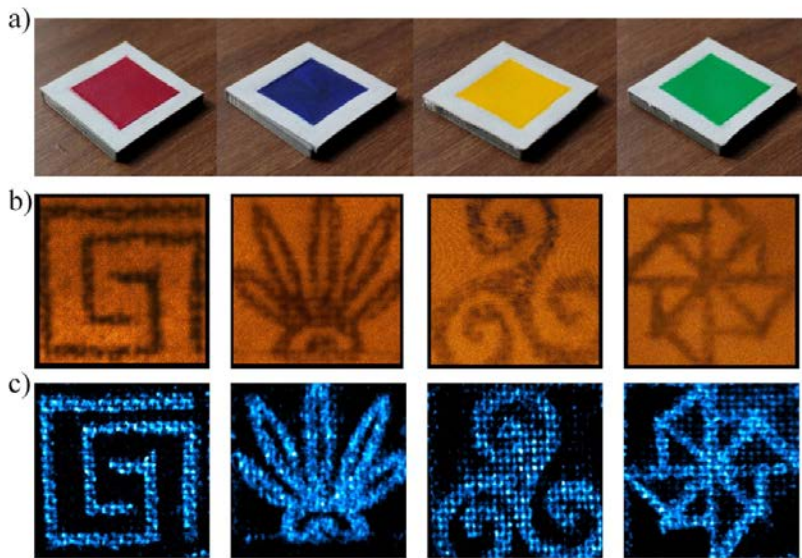
Fig. 8. a) Bright-field images of the four canvas samples; b) underdrawing visualization through Spectral-OCT (images size 9 \times 9 \text{ mm}^2 , sampling step of 5 \text{ }\mu\text{m} on x and y, and 3.55 \text{ }\mu\text{m} on z); c) NIR photoacoustic imaging (scanning area: 10 \times 10 \text{ mm}^2 , 750 averaging measurements per point).
