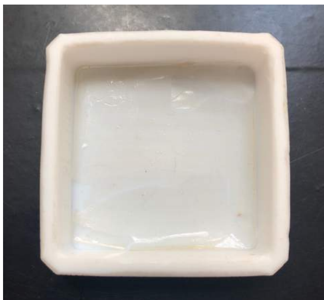
Figure 3.2 Animal glue was dried on a Teflon hold to form a film for spectra collection.
