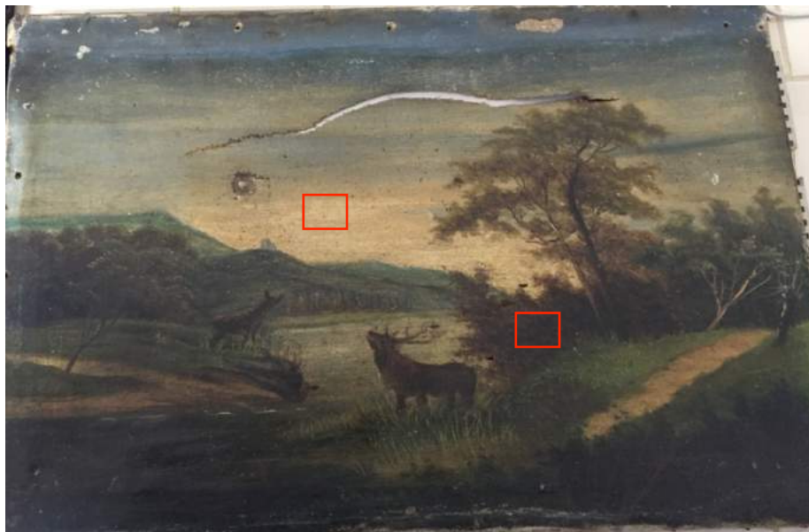
Figure 5.1 The old painting used for the validation of the hyperspectral sensor ASD FieldSpec FR Pro as non-invasive and non-destructive method of pigments and binding medium characterization.
