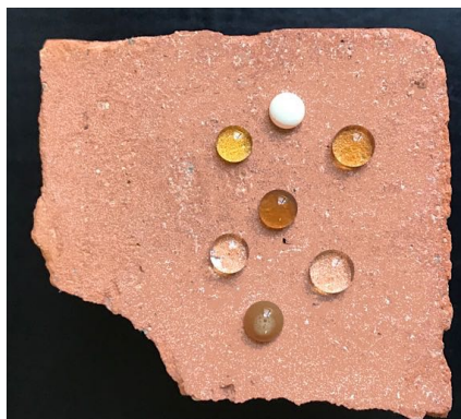
Figure 4.18 Digital photo of water, black tea, olive oil, coffee and milk drops in contact with coated red brick. All drops are quasi spherical and this spherical shape is stable over time.
