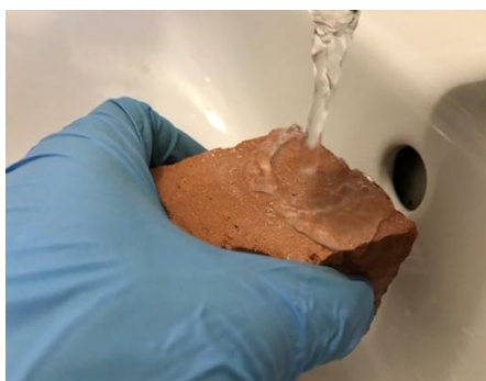
Figure 4.19 Digital image of coated red brick under running tap water. The surface maintained completely dry and water rolled off.
