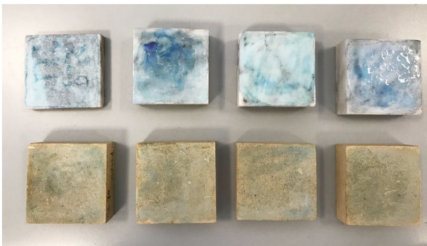
Figure 5.1 MB stained and then water sprayed samples ready for UV radiation.
