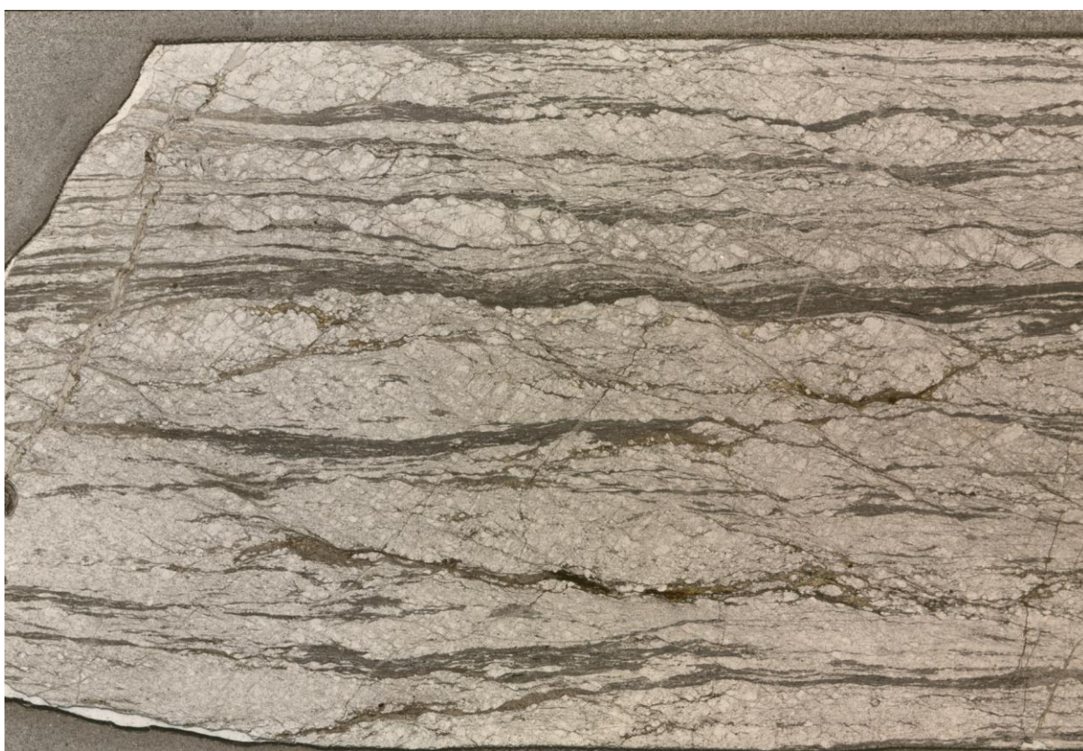
Figure D5 – Photo scan of thin section SP78 (Praticciolo) used for the analysis of the orientations of the Sm foliation and C' shear bands (see Chapter 5).
