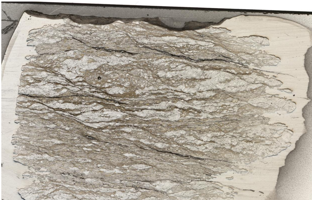
Figure D2 – Photo scan of thin section CS30 (Praticciolo) used for the analysis of the orientations of the Sm foliation and C' shear bands (see Chapter 5).
