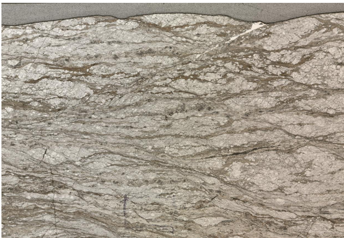
Figure D3 – Photo scan of thin section SP65 (Praticciolo) used for the analysis of the orientations of the Sm foliation and C' shear bands (see Chapter 5).
