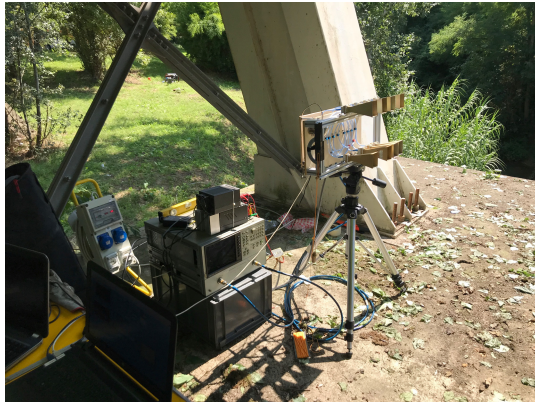
Fig. 12. Photograph of the radar installation.
