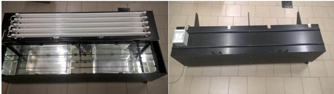
Figure 5.1. Light-induction chamber for freely moving and fully awake mice. Rod degeneration is induced upon a short, high intensity illumination.
