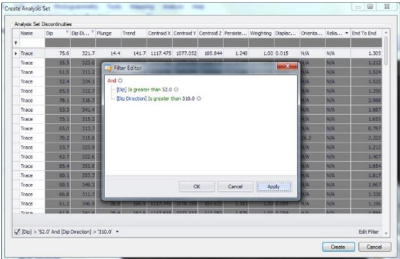
Figure 24- Selection of filter parameter to extract the sets of discontinuities by SiroJoint
