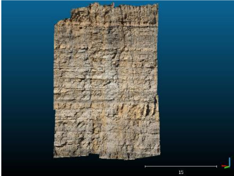
Figure 72 - 3D model carried out with the stereo pairs of the highwall nr 2
