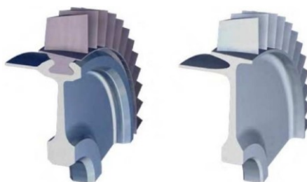
Figure 230 The two ways to obtain a turbine rotor: hub and blades assembly (left) and blisk (right) (from [83])
