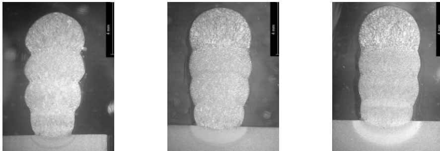
Figure 26 Effect of the interpass temperature on the cross section of a wall. Interpass temperature increasing from left to right (from [16])
