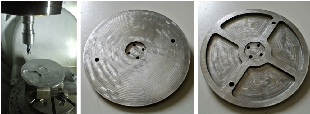
Figure 174 Milling of the C axis table (left) and final result (center and right)
