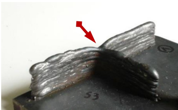
Figure 89 The big deposition failure (pointed by the red arrow) in one of the specimens manufactured using the S3 deposition strategy
