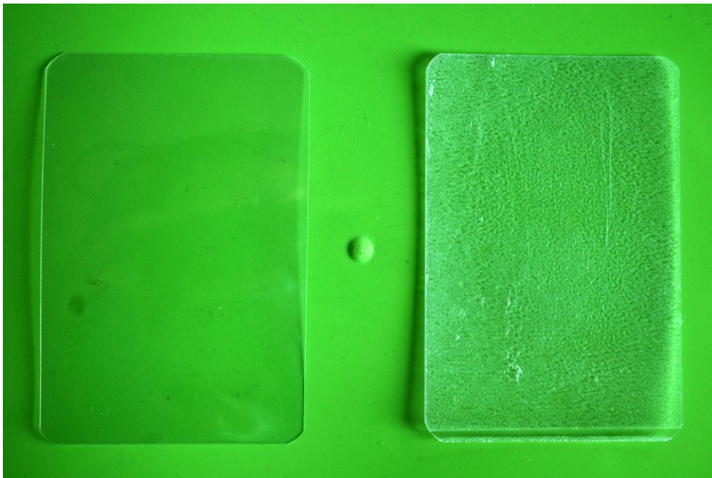
Figure 306 The PET sheet used to manufacture the lens for the speckle before (left) and after it has been impressed with a P600 sheet of sandpaper (right)
