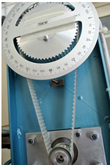
Figure 196 A picture taken during the determination of the steps/degree ratio for the C axis
