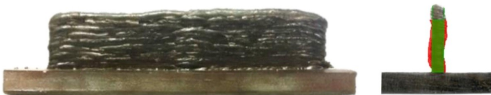
Figure 21 A wall manufactured using WAAM and its cross section (in green the final wall after machining, in red the zones to be machined away)
