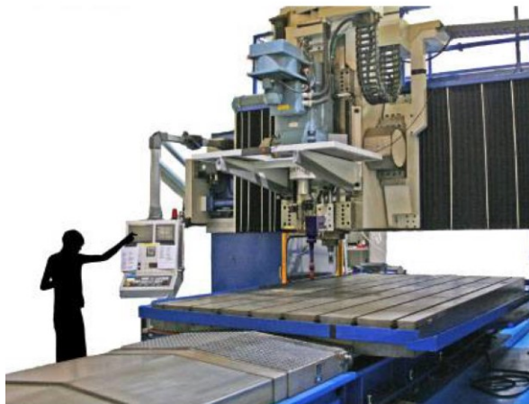
Figure 123 The machine obtained by Cranfield university through the retrofit of a former friction stir welding machine (from [8])
