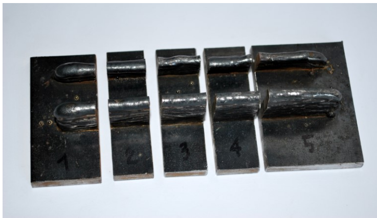
Figure 54 One of the manufactured walls divided in five parts to measure the surface waviness
