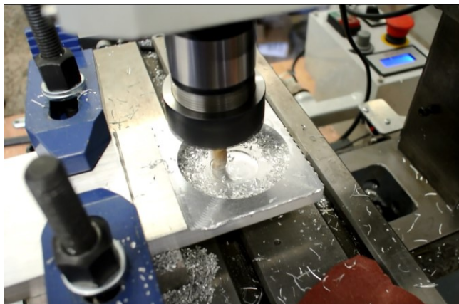
Figure 172 Milling of one of the bearing supports
