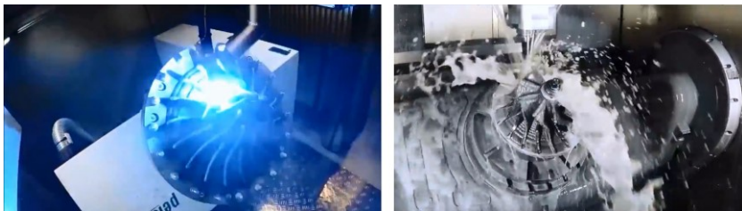
Figure 215 Impeller manufactured using WAAM technology (left) and its post finishing operation (right) (source: Gefertec)
