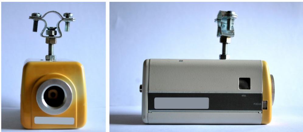
Figure 309 Front view (left) and side view (right) of the pattern projector assembly
