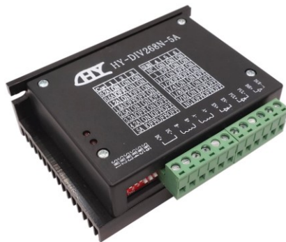
Figure 141 The HY-DIV268N-5A driver used to control the motors of the linear axes
