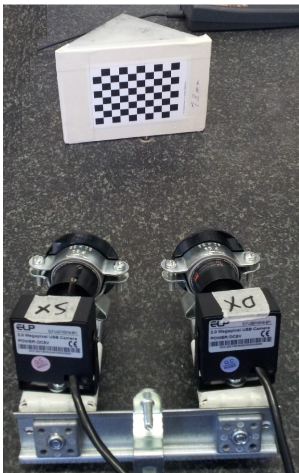
Figure 304 The two cameras mounted on the support and placed in front of the prism for the calibration procedure
