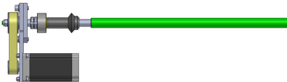
Figure 137 General configuration of the motor and screw (green element) for a linear axis of the machine. The yellow element in the picture is the toothed belt
