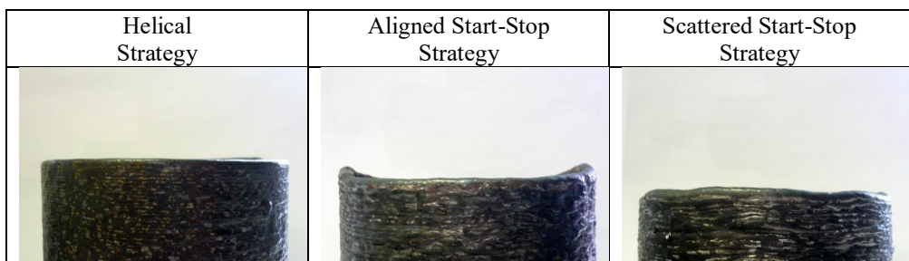
Figure 105 Top surfaces for three different tubulars manufactured with the three presented deposition strategies
