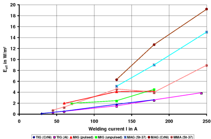
Figure 282 Correlation between welding current and total emission (from [100])
