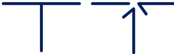
Figure 100 The new deposition strategy proposed by the Authors for T-Crossings. The original curves from the “First Layer Curve List” (left) and the toolpath optimized for the T Crossing (right)
