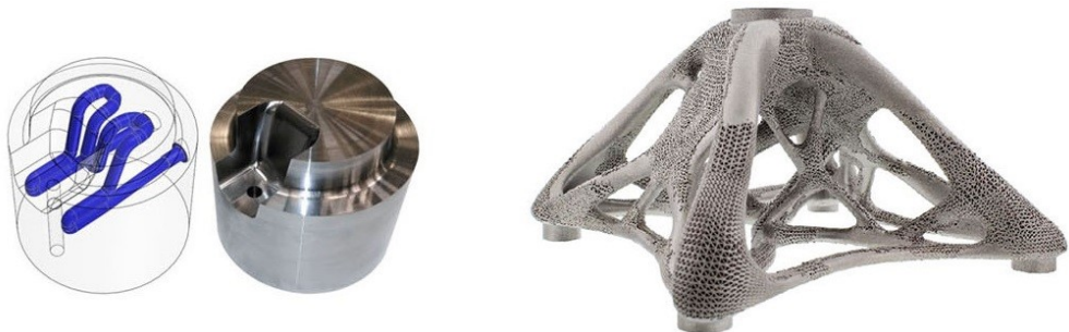
Figure 33 An example of conformal channels for a mold (left) (from [26]) and of lightweight lattice structure (right) (from [27]). Both these parts must be manufactured using powder bed techniques
