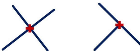
Figure 71 In the CAD skeleton representation, each crossing feature is represented with a point located in the intersection of the surfaces composing the feature itself
