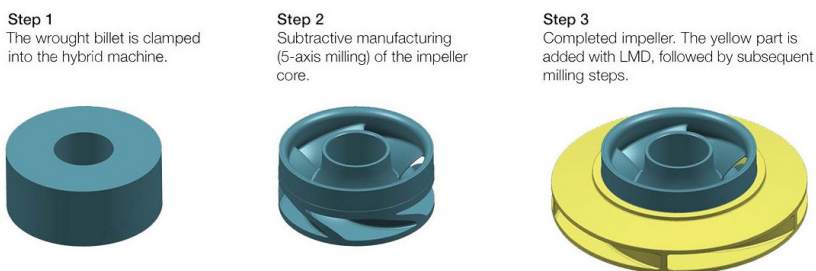
Figure 217 Hybrid building procedure for a shrouded impeller (from [82])
