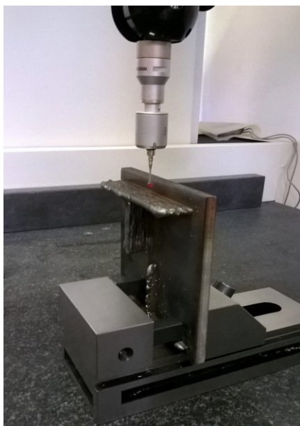
Figure 95 The acquisition of the back surface of one of the manufactured specimens in the CMM machine
