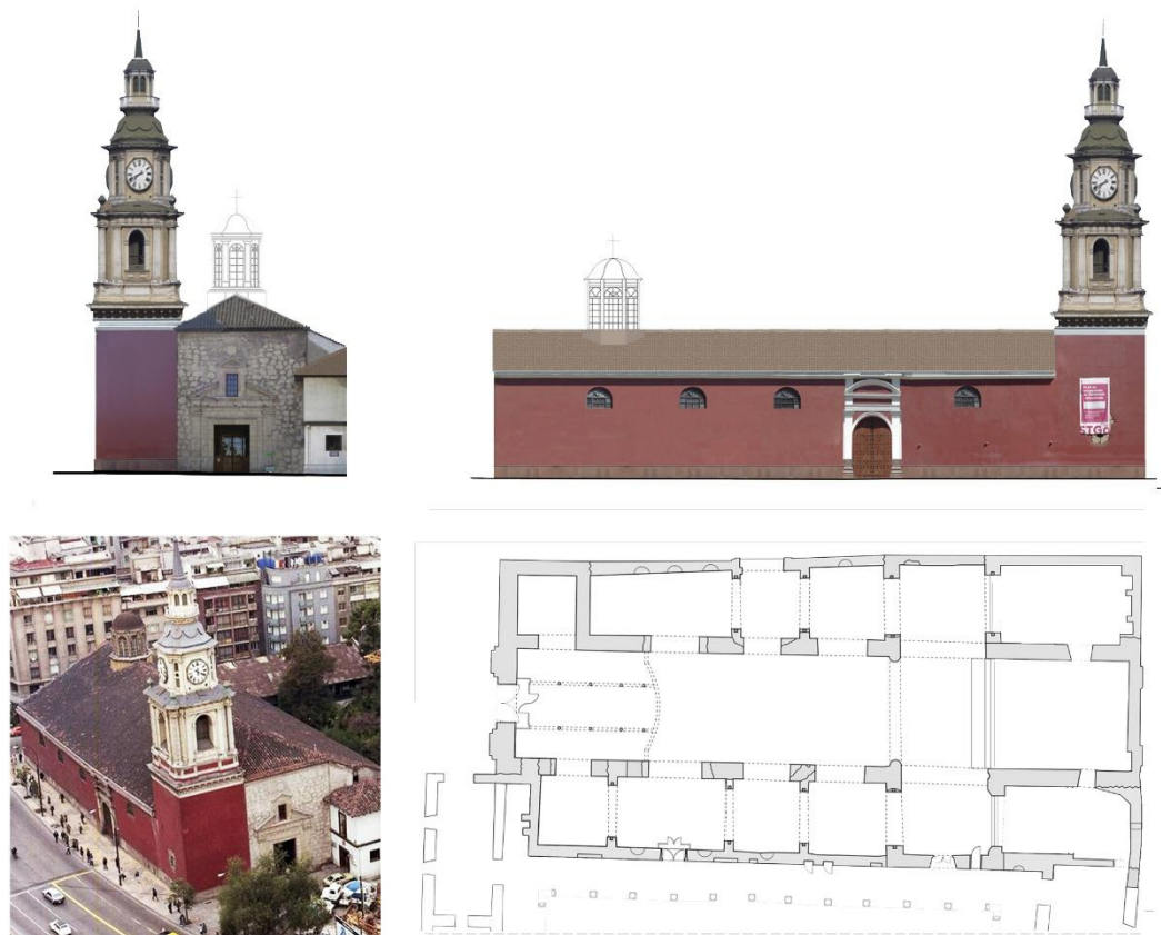
Figure 5.2.1 - View of the façade, current plan, façade and section of the San Francisco church.
