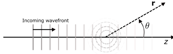
Figure 1.1: Sketch of the scattering process within the center of mass frame: a fictitious particle of mass \mu (reduced mass) impacts on a fixed scatterer potential. The amplitude of the scattered wavefront is determined by the scattering amplitude f as a function of the scattering angle \theta .
