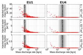
Fig. 1. Injected water mass fraction versus MDR as a function of aquifer permeability (k). Detailed information is presented in Supplementary Material.
