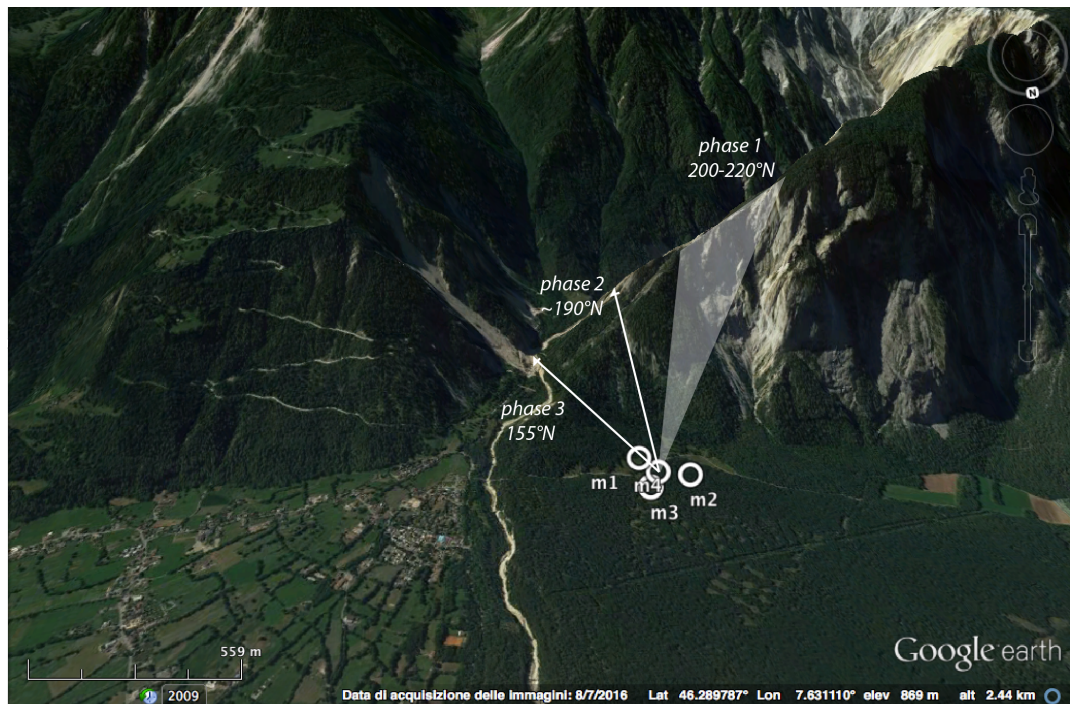
FIGURE 4.5: Google-earth projection of back-azimuth of the three phases identified from infrasound back-azimuth during the initiation of the May 29, 2017 event and highlighted in Figure 4.1.
