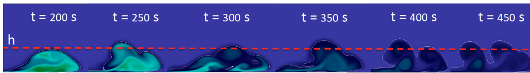
FIGURE 5.13: Six time snapshots of the head of the current with a solid particles concentration decreasing with time because of the entrainment process (see colorbar of Fig.5.11). The red dashed line represent the initial height of the 2D volume, h .
