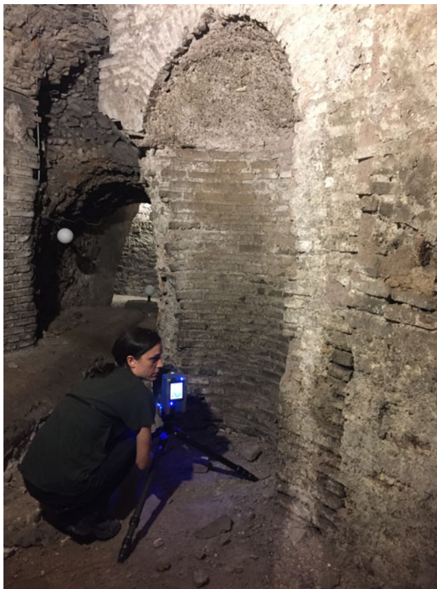
Fig. 1. Beatrice Fochetti sets up the FARO Focus laser scanner prior to recording the Nymphaeum in SGL2 Area 1 (Stephen Kay)
