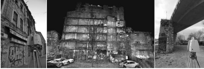
Figure 6. 3D Laser Scanning in Beyoğlu to Create the Bases for a Detailed Digital Twin of the Urban Façade of the Neighborhood (March 2019).
