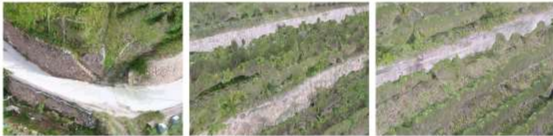
The the final mesh allowed to classify and measure the types of retaining wall. From left to right: drywall, exposed stone façade, reinforced concrete wall.
