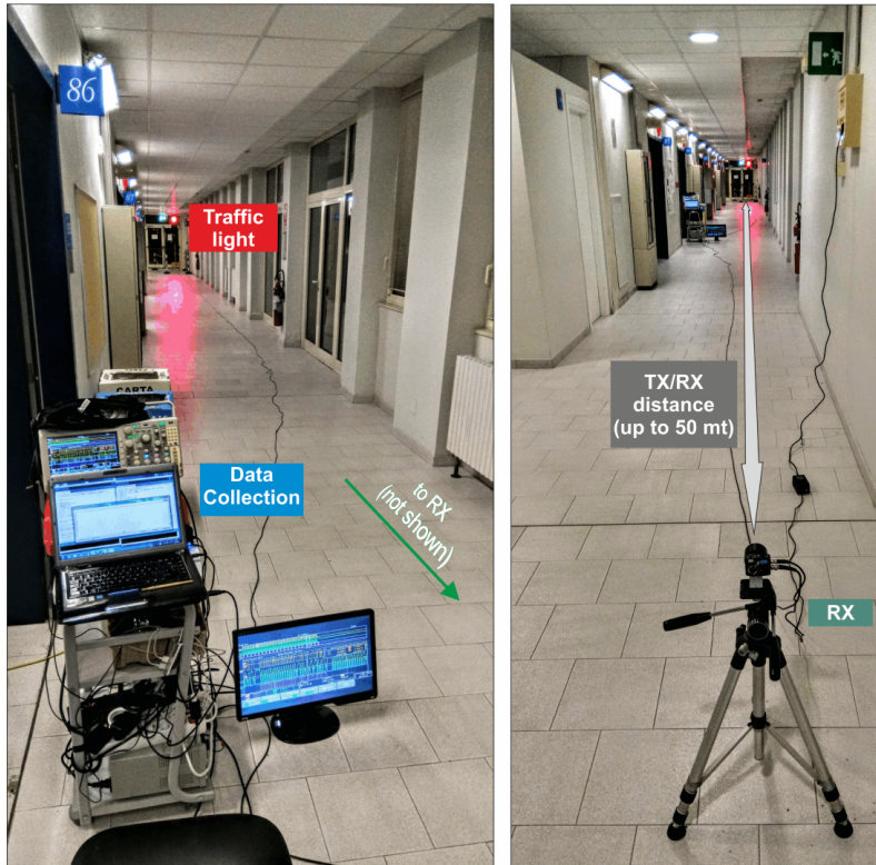
Figure 3.23: Experimental campaign: a standard traffic transmits VLC signal to a photo-receiver stage equipped with digital Active Decode and Relay block. The data collection unit consists of a PC and an oscilloscope. The distance between transmitter and receiver is up to 50 m limited by available line of sight length in the building.
