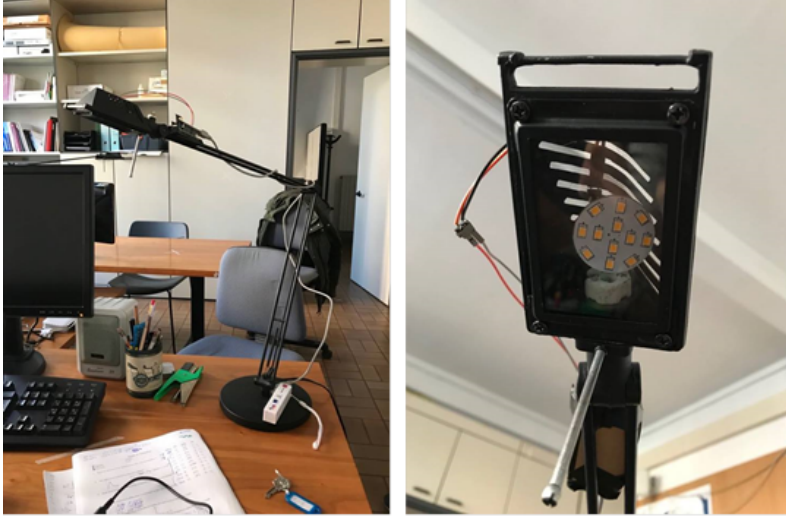
Figure 4.1: Table lamp modified for VLC Light.
