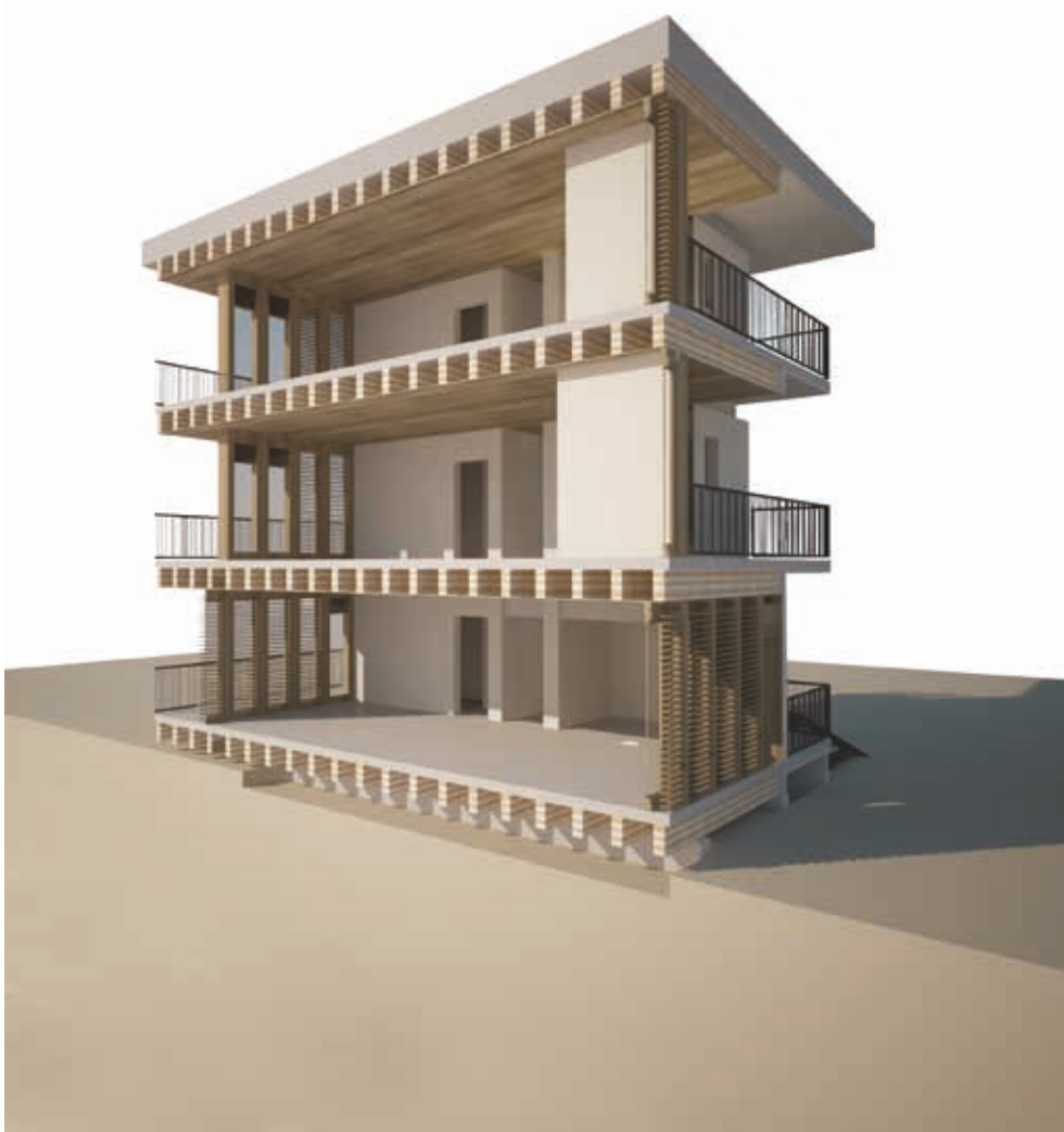
Figure 10. A sectional perspective of the structure of the S.A.T.O.R. Project virtual prototype illustrating the balloon frame construction system of the living space unit.
