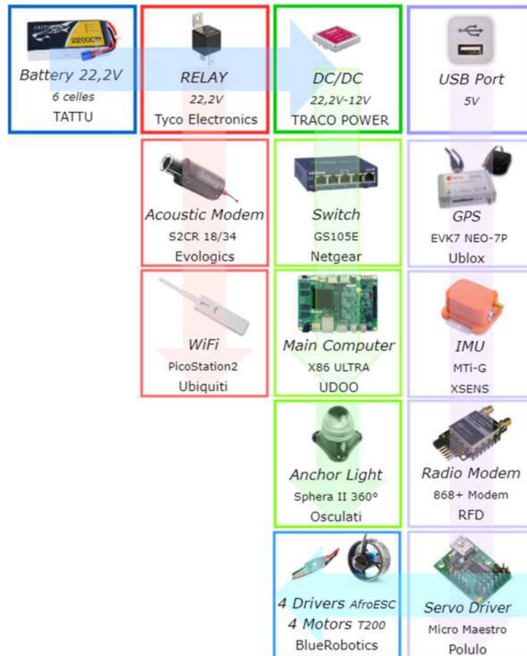
Figure 4.4: Power supply scheme.
