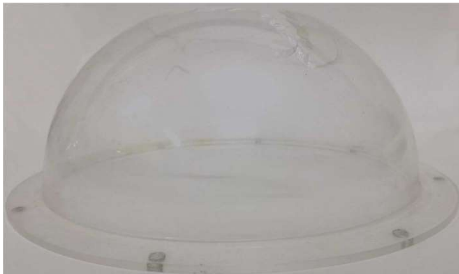
Figure 3.6: Check of breaking mode, first buckling example.
