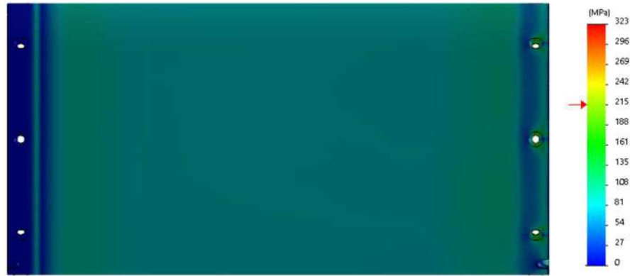
Figure 4.18: Static analysis results, stresses; (cylinder lateral view).
