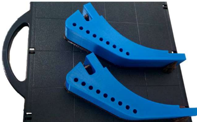
Figure 2.4: Rear thrusters ABS supports.
