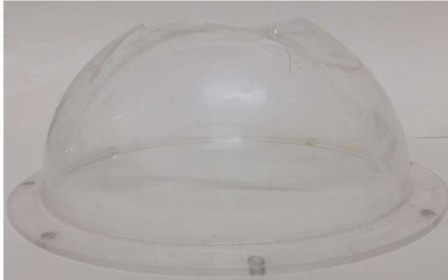
Figure 3.7: Check of breaking mode, second buckling example.
