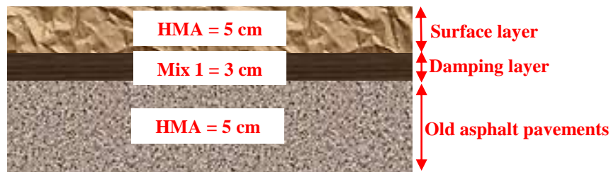
Figure 6.20 Pavement structure with a damping layer
