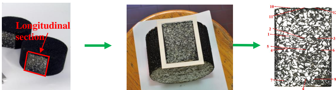
Figure 6.13 Longitudinal section of the HWT sample
