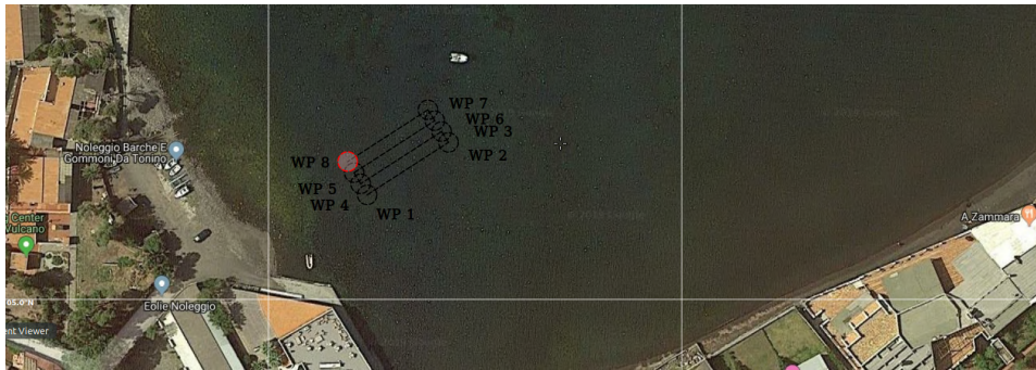
Figure 5.14: Google Earth image of the Negro Bay, Vulcano Island (Italy) overlaid with the planned autonomous underwater mission. The waypoints are indicated with WP.
