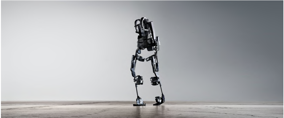
Figure 1.2: An example of an assistive robotic device. The figure shows a lower limb exoskeleton designed to assist people with motor disability during the gait.
