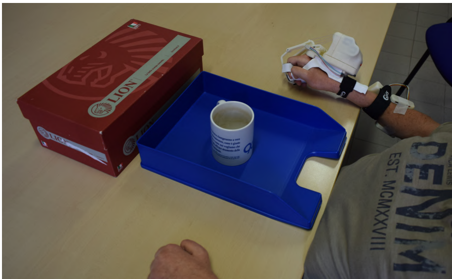
Figure 4.7: An example of the test scenario: the subject is seating in front of a blue dais and a shoe box, in the center of the blue dais one of the test objects (in this case an empty mug) is placed, such object that must be moved over the shoe box, and the action shall be carried out using only the upper right limb on which the HES has been previously mounted.
