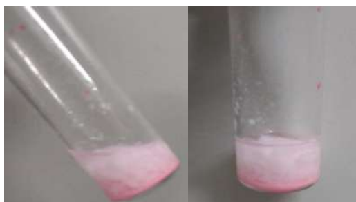
Figure 4.2 (c). Systems obtained from the reaction between PNIPAM and PMMA microgels swollen in EtOH/water mixtures after 4 hours.
