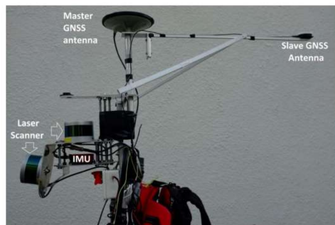
Figure 1. In-house-built backpack laser scanner.
