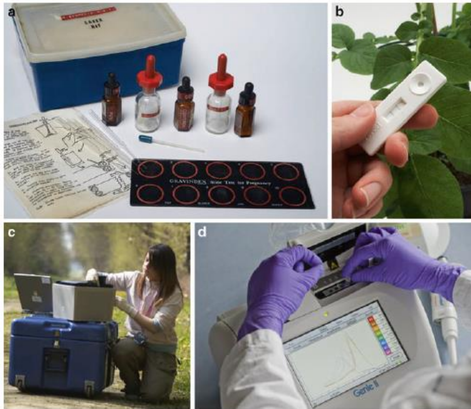
Figure 4: field diagnostics tools based on a) Latex agglutination b) Lateral flow devices kit c) Portable PCR d) Isothermal AMPlification reaction test. Credits: Boonham et al. , 2014
