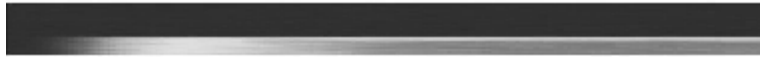
Fig. 7. Absorber image for N-S misalignment of the whole system \beta=0.5^\circ (in Dec.).
